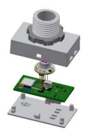
Assemble PCB assembly into housing as shown.
