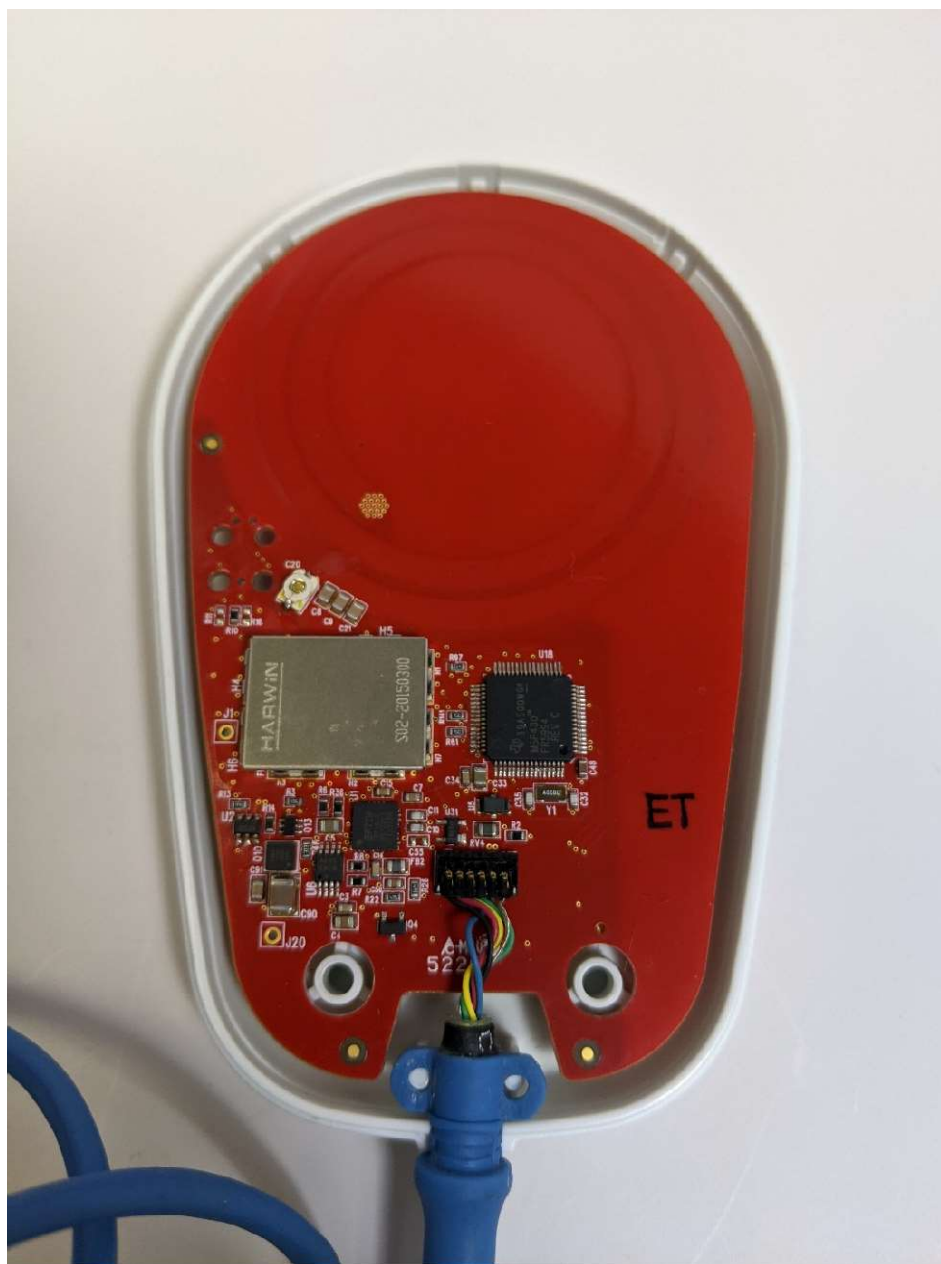
Internal Picture 5: Bottom PCB with shield over amplifier circuitry.
