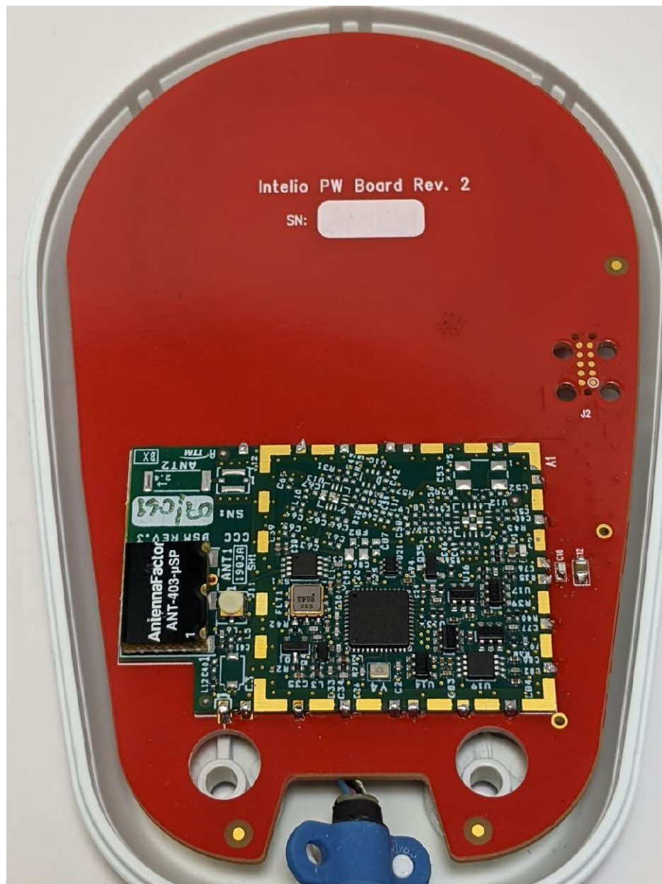
Internal Picture 2: Top PCB layout of the Intelio Programming Wand, with attached BSM07 RF Communication module for MICS operation.
