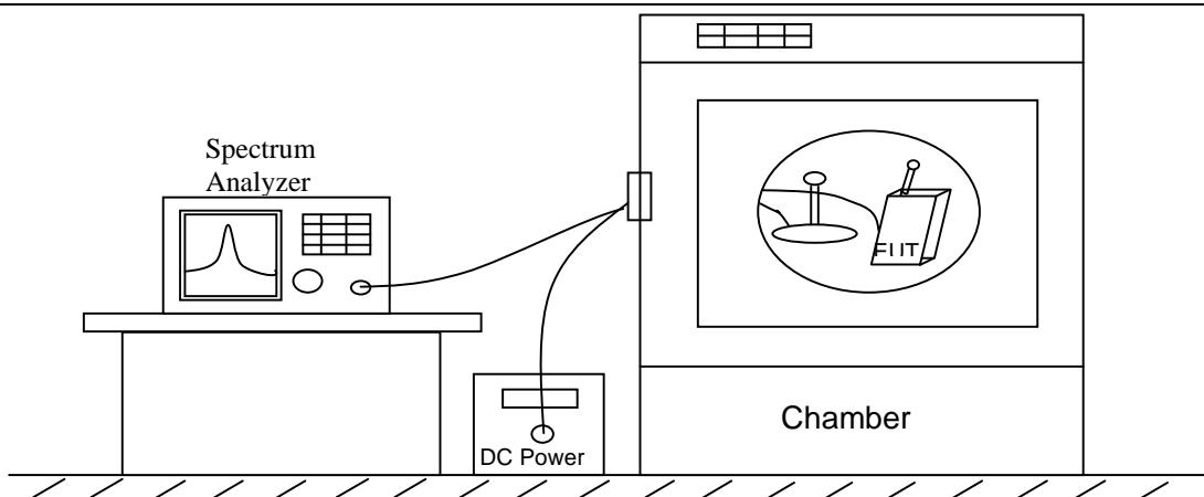
***Frequency stability measurement configuration***
