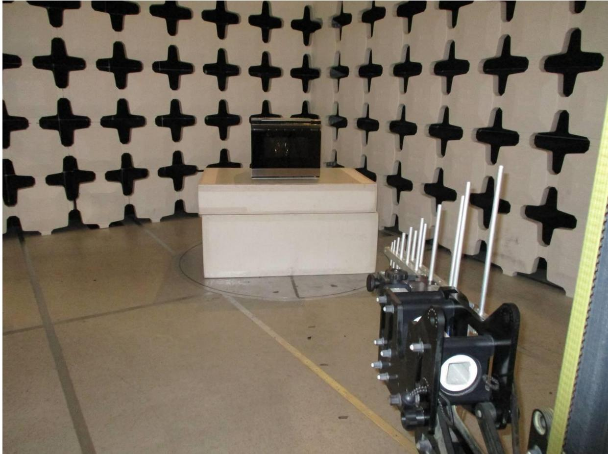
**Figure 3. Radiated Emissions Measurement Photo, 200 to 1000 MHz (both Power Supplies)**
