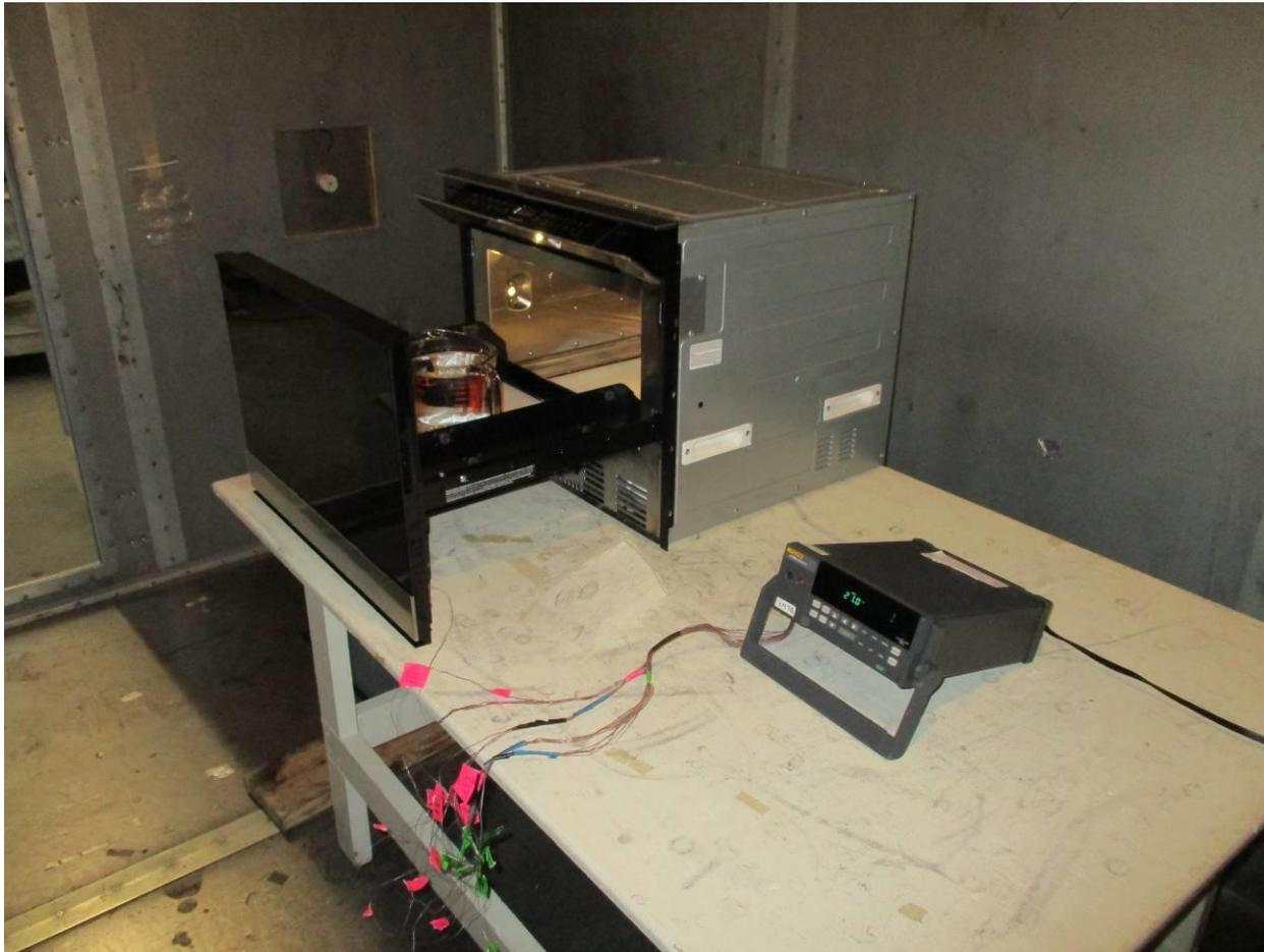
**Figure 5. Output Power Test Configuration (both Power Supplies)**
