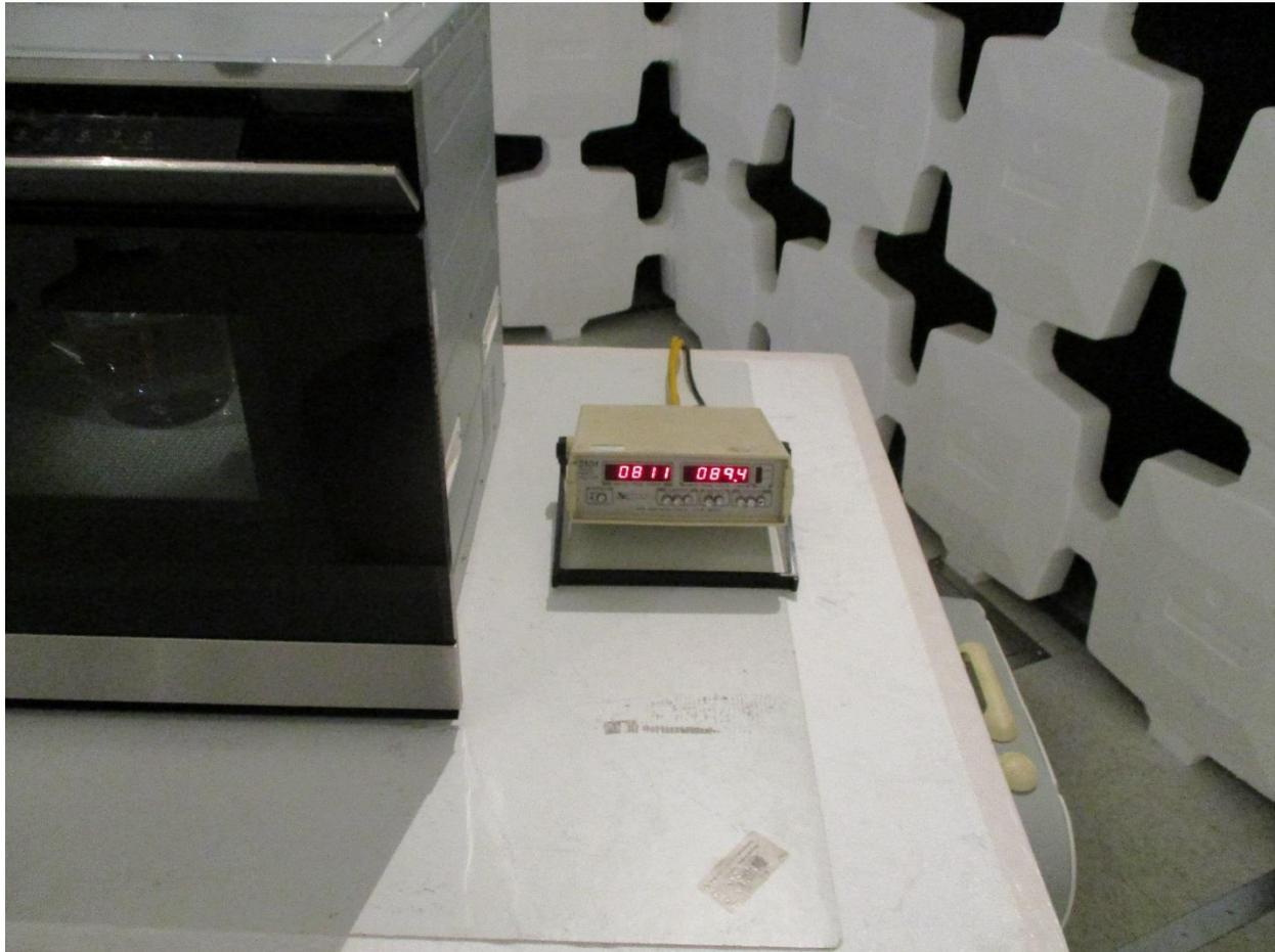
**Figure 6. Input Power Test Configuration (both Power Supplies)**
