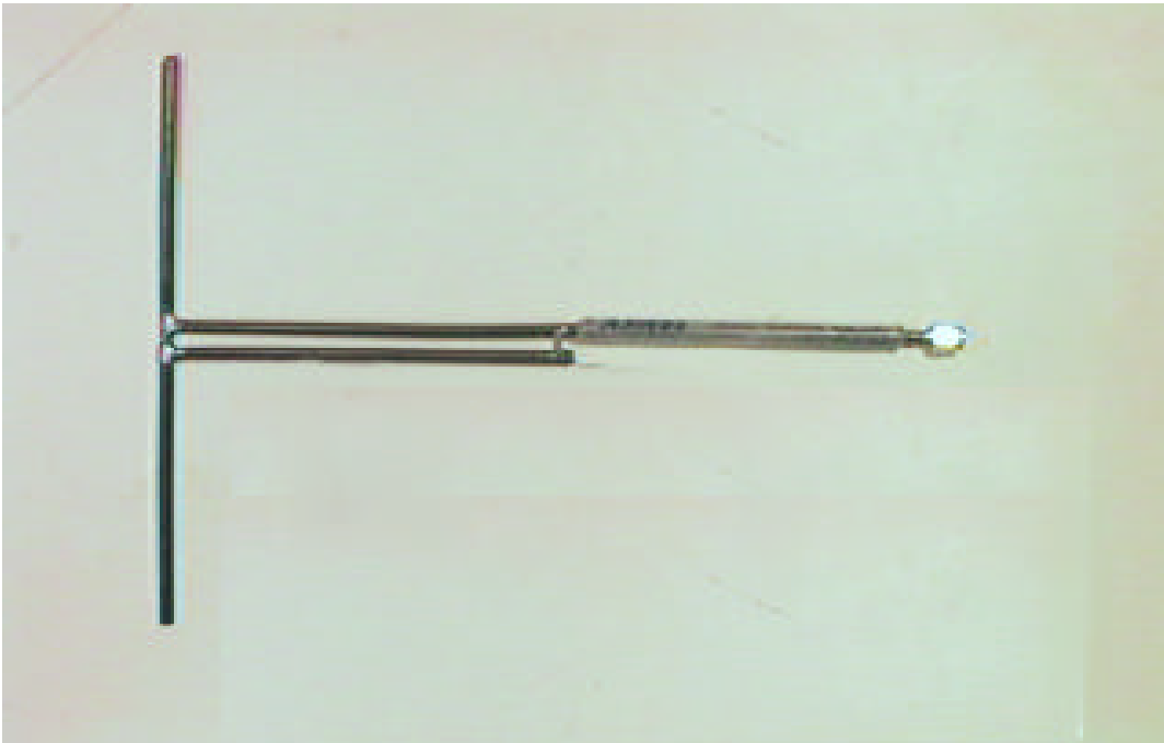
Reference Dipole Antenna Used for ERP Measurement
