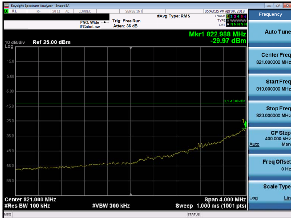
Plot 7-136. Lower Extended Band Edge Plot (Band 26/5 - 1.4MHz QPSK - Full RB Configuration)
