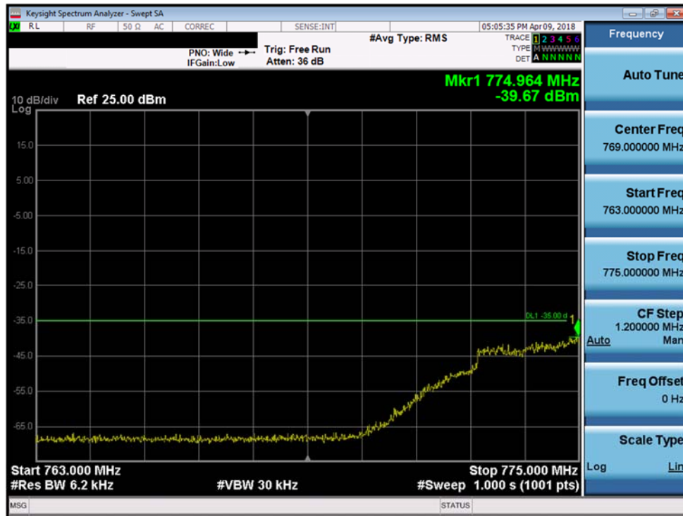
Plot 7-128. Lower Emission Mask Edge Plot (Band 13 - 5.0MHz QPSK - Full RB Configuration)
