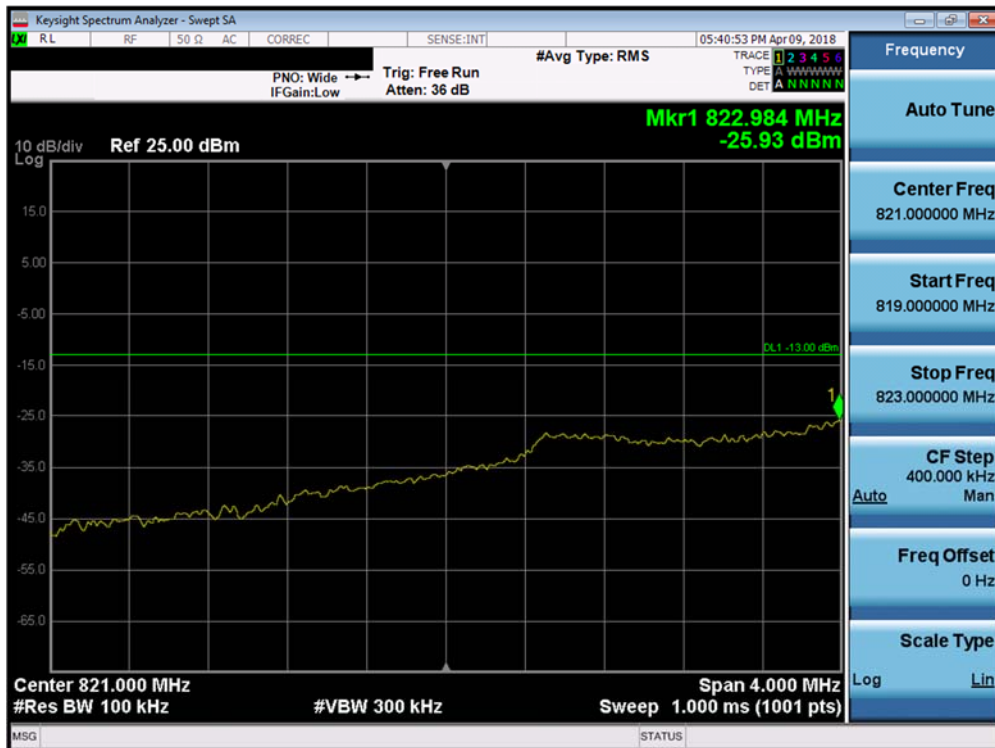
Plot 7-140. Lower Extended Band Edge Plot (Band 26/5 - 3.0MHz QPSK - Full RB Configuration)
