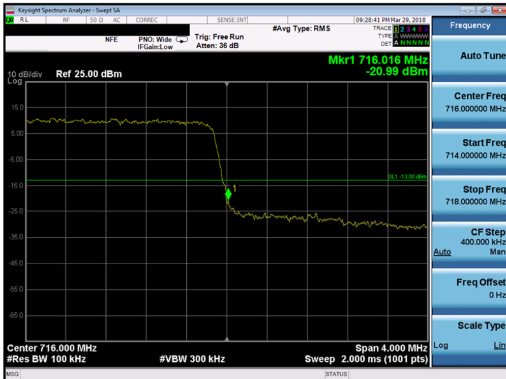
Plot 7-120. Upper Band Edge Plot (Band 12 - 3.0MHz QPSK - Full RB Configuration)
