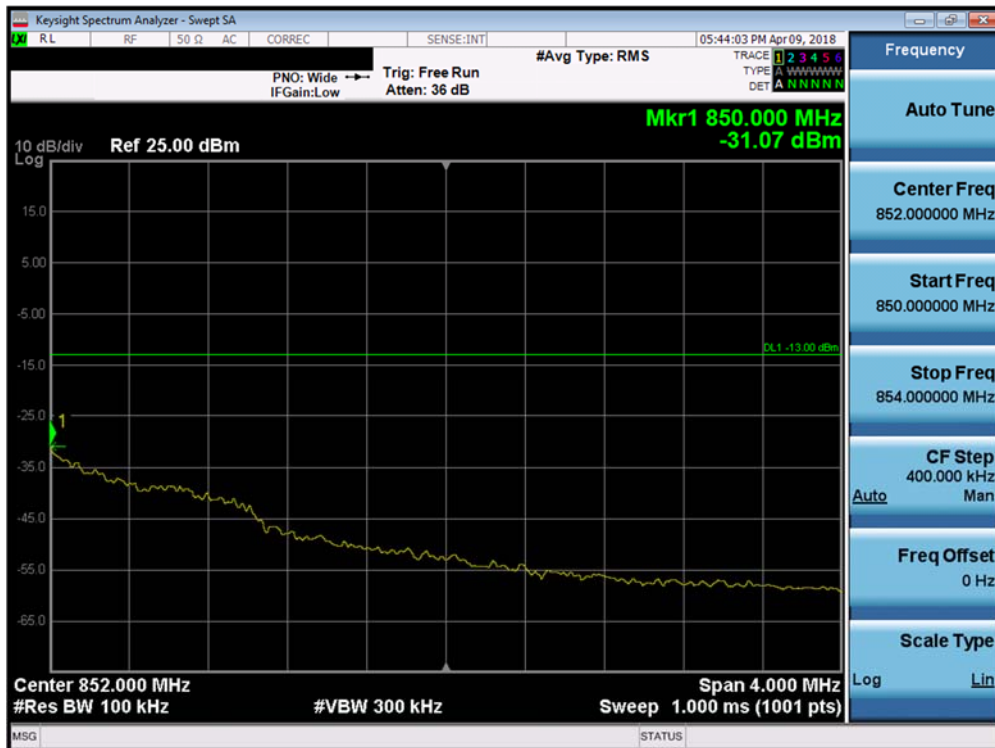
Plot 7-138. Upper Extended Band Edge Plot (Band 26/5 - 1.4MHz QPSK - Full RB Configuration)
