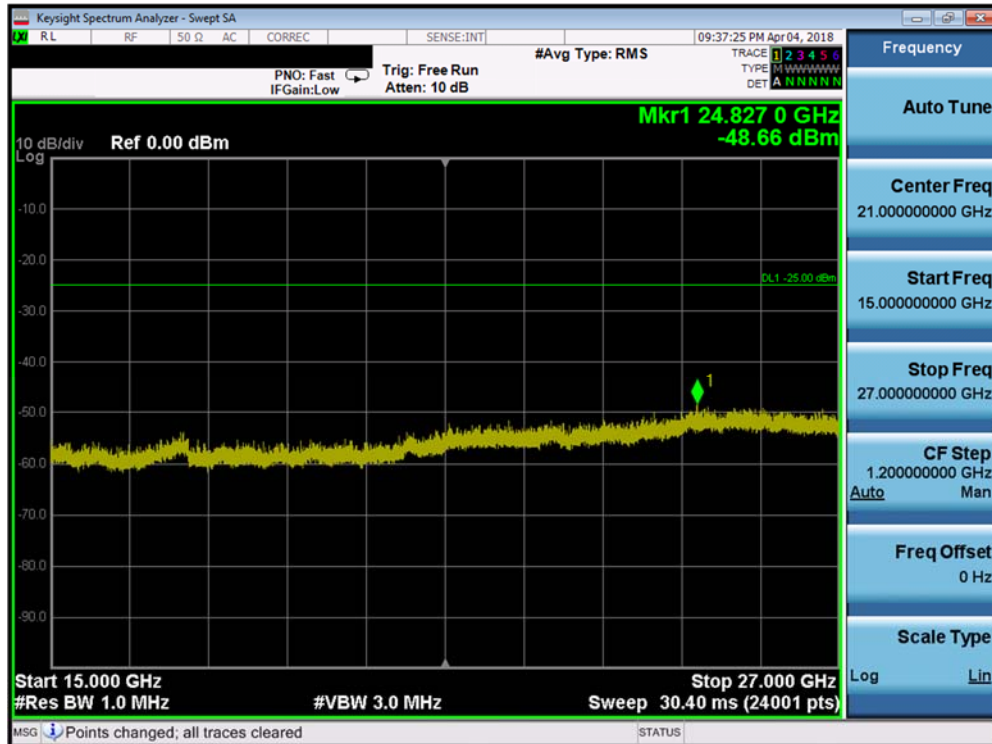
Plot 7-113. Conducted Spurious Plot (Band 41 PC2 - 20.0MHz QPSK - RB Size 1, RB Offset 0 - Mid Channel)
