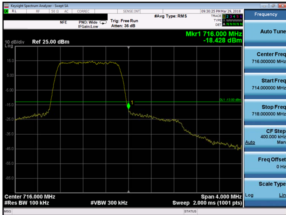
Plot 7-118. Upper Band Edge Plot (Band 12 - 1.4MHz QPSK - Full RB Configuration)
