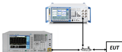
Figure 7-3. Test Instrument & Measurement Setup
