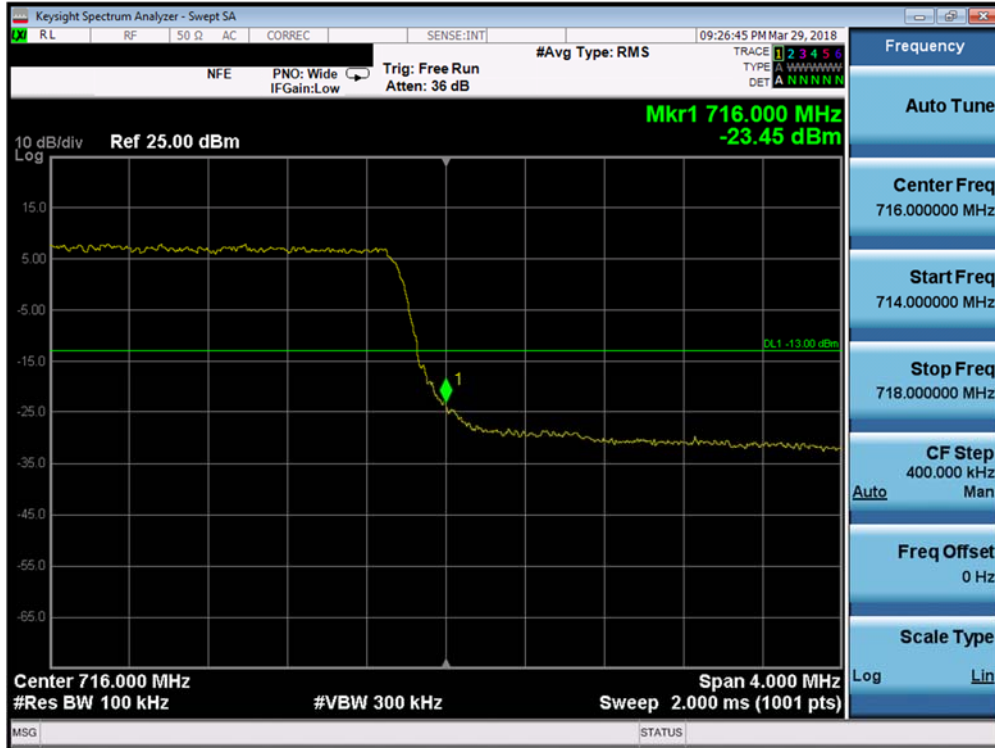
Plot 7-123. Upper Band Edge Plot (Band 12/17 - 5.0MHz QPSK - Full RB Configuration)
