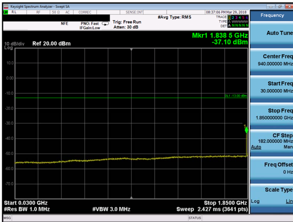
Plot 7-102. Conducted Spurious Plot (Band 25/2 - 20.0MHz QPSK - RB Size 1, RB Offset 0 - Mid Channel)
