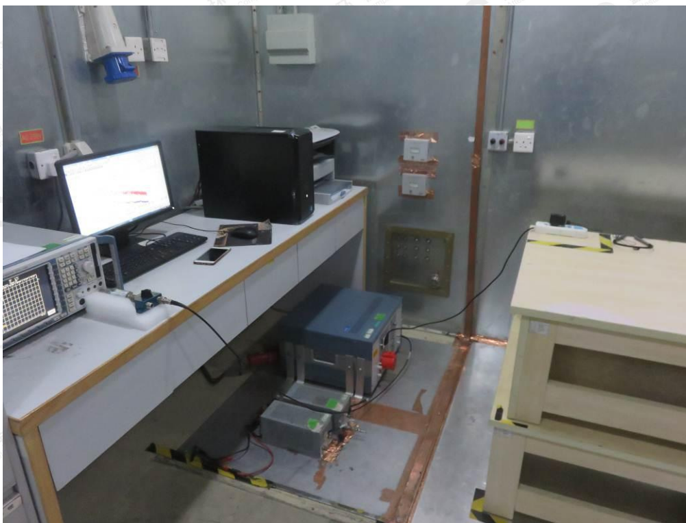
FCC RADIATED EMISSION TEST SETUP
