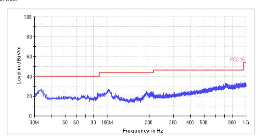
The emission levels with 960 to 1000 MHz also comply with the ICES-005 limit 46 dB $\mu$ V/m. All emission levels are more than 6 dB below the limit.
