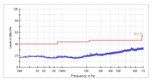
The emission levels with 960 to 1000 MHz also comply with the ICES-005 limit 46 dB $\mu$ V/m. All emission levels are more than 6 dB below the limit.
