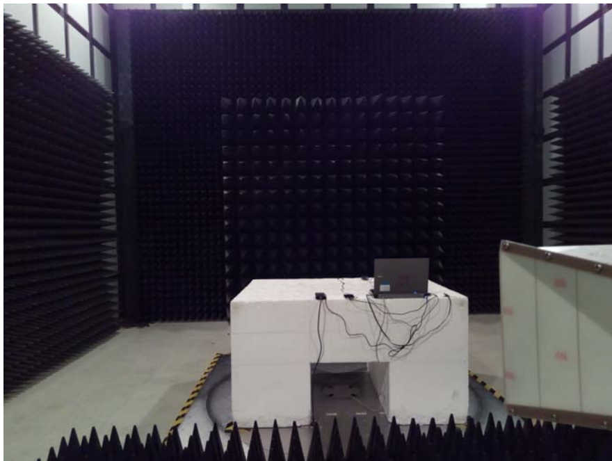
Radiated Emissions – Rear View (Above 1 GHz)
