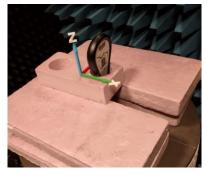
Radiated Power at 2405 MHz, TRP = -8.75 dBm, Max EIRP = -3.31 dBm
