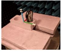
Radiated Power at 2475 MHz, TRP = -10.44 dBm, Max EIRP = -5.25 dBm
