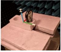
Radiated Power at 2445 MHz, TRP = -9.78 dBm, Max EIRP = -4.54 dBm
