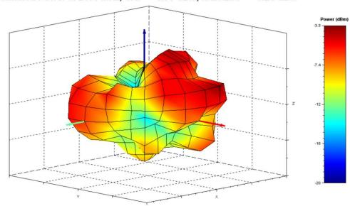
Radiated Power at 2405 MHz, TRP = -8.75 dBm, Max EIRP = -3.28 dBm
