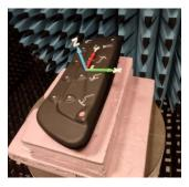
Radiated Power at 2475 MHz, TRP = -12.39 dBm, Max EIRP = -6.58 dBm
