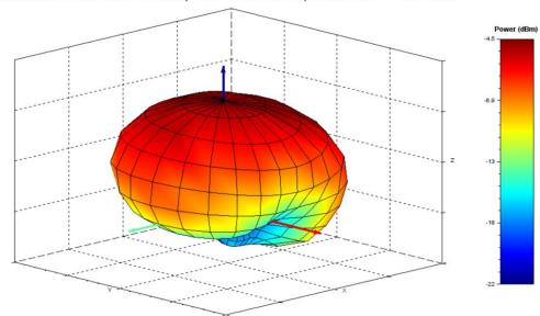
Radiated Power at 2445 MHz, TRP = -9.78 dBm, Max EIRP = -4.54 dBm
