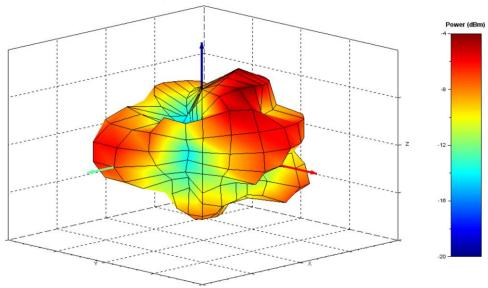
Radiated Power at 2445 MHz, TRP = -9.61 dBm, Max EIRP = -4.04 dBm
