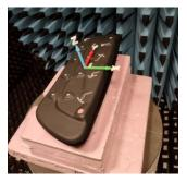
Radiated Power at 2405 MHz, TRP = -8.75 dBm, Max EIRP = -3.28 dBm
