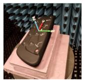
Radiated Power at 2445 MHz, TRP = -9.61 dBm, Max EIRP = -4.04 dBm
