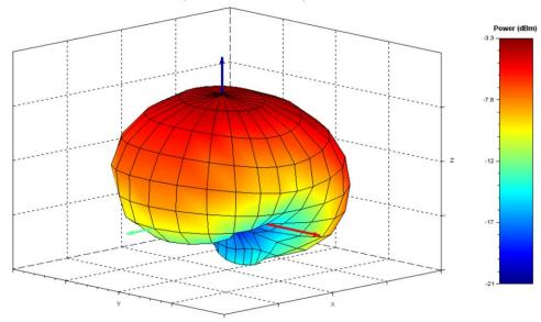
Radiated Power at 2405 MHz, TRP = -8.75 dBm, Max EIRP = -3.31 dBm
