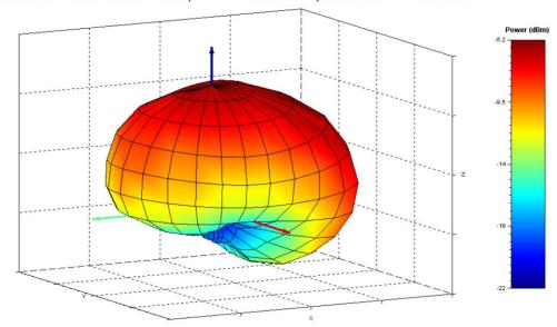
Radiated Power at 2475 MHz, TRP = -10.44 dBm, Max EIRP = -5.25 dBm
