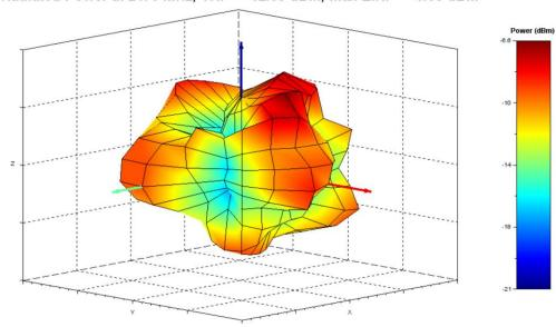
Radiated Power at 2475 MHz, TRP = -12.39 dBm, Max EIRP = -6.58 dBm
