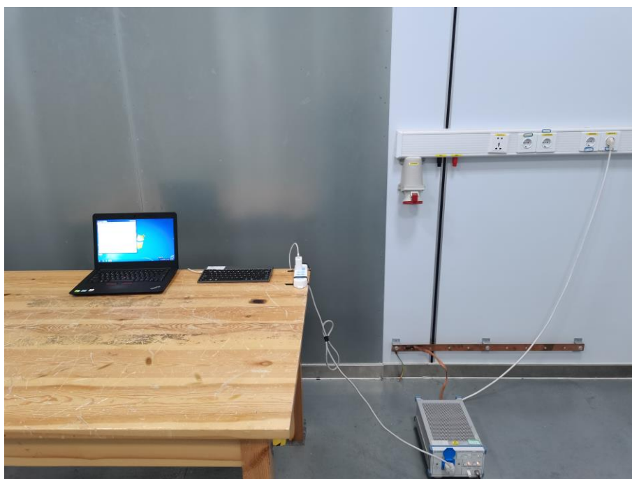
Fig. 4 Power line conducted emission setup photo
