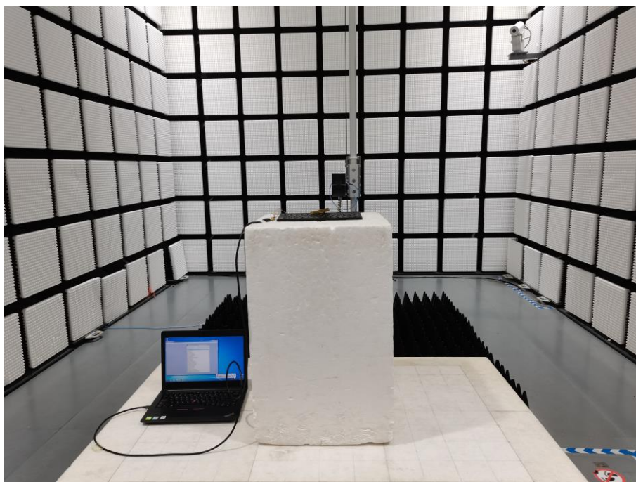
Fig. 3 Radiated emission setup photo(Above 1GHz)
