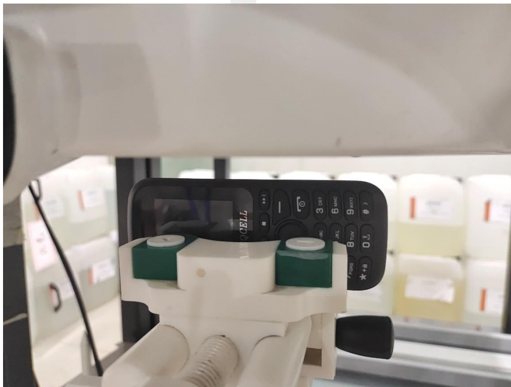
Body Right side(separation distance is 10mm)
