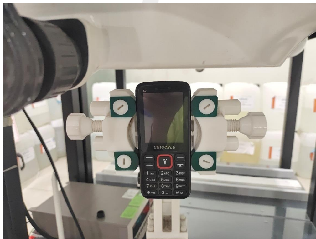
Body Top side(separation distance is 10mm)
