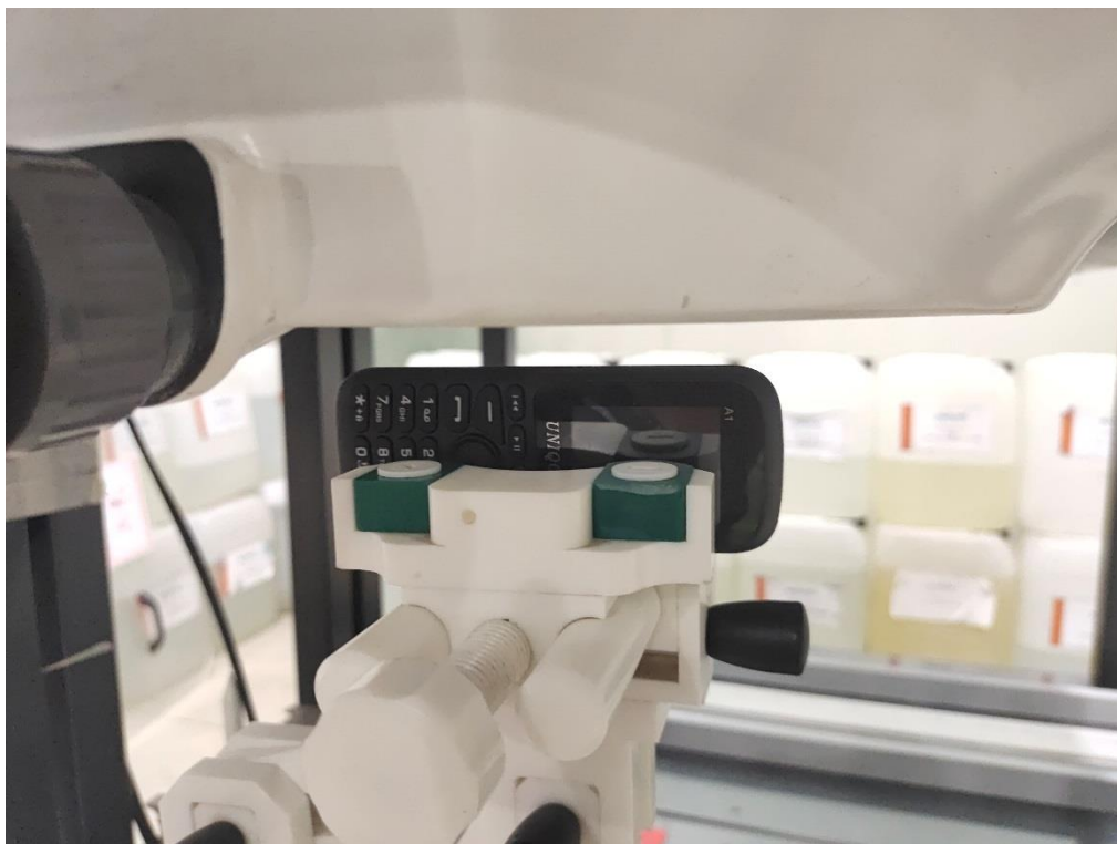
Body Left side(separation distance is 10mm)
