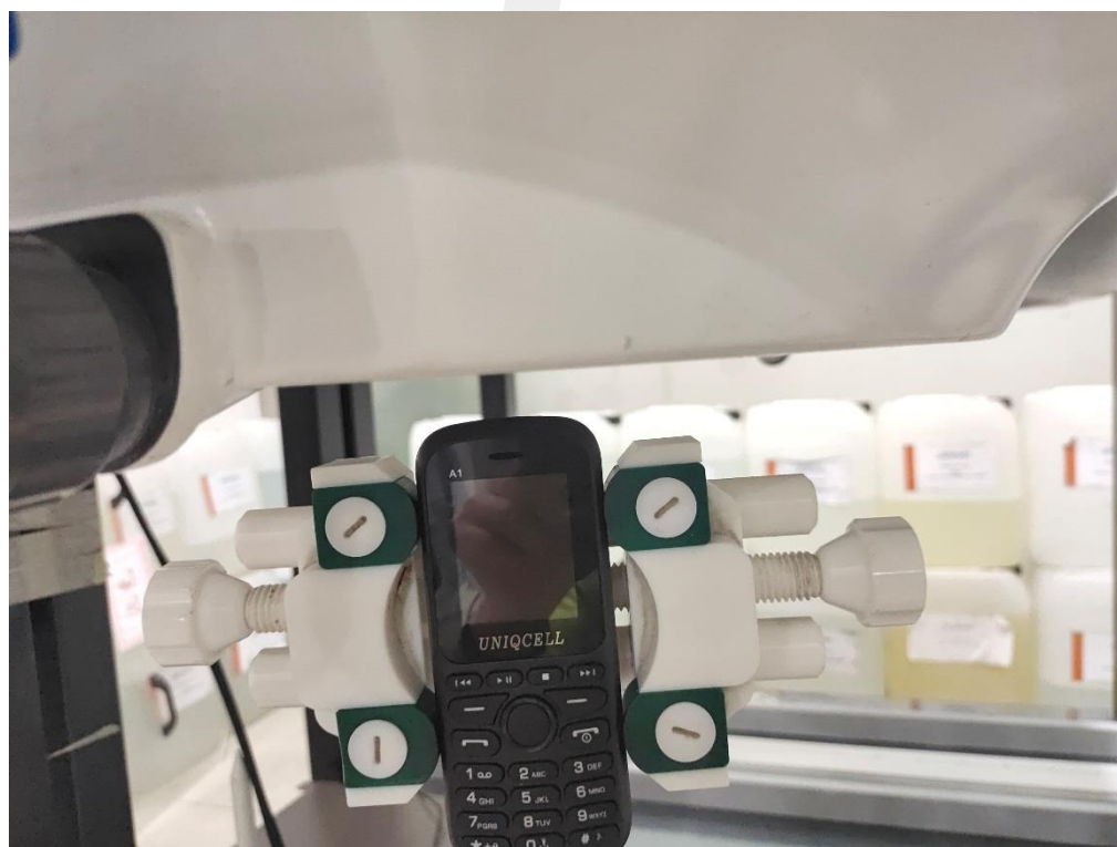
Body Top side(separation distance is 10mm)
