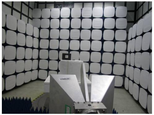
1.3 Radiated Spurious Emissions Test Setup
