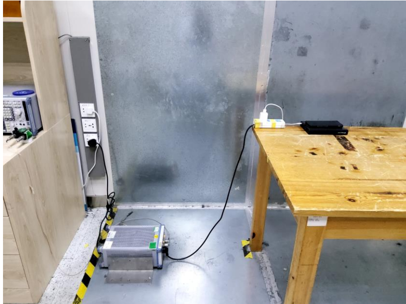
Radiated Spurious Emissions Test Frequency From 9KHz-30MHz
