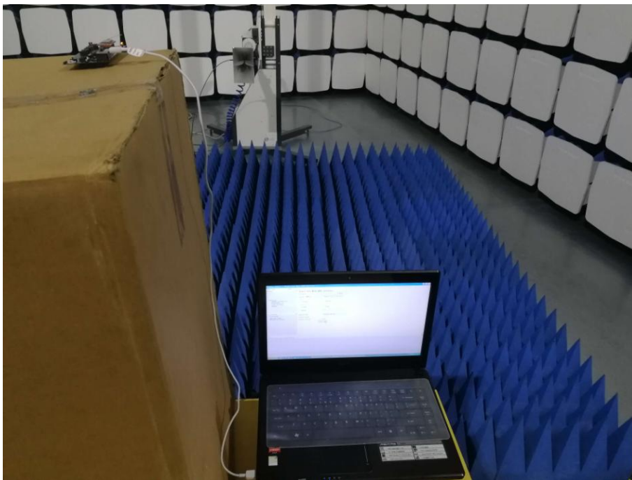
Test Mode_1 - Radiated Emission test view (Frequency above 1GHz)
