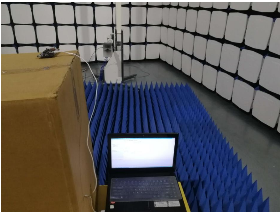
Test Mode_3 - Radiated Emission test view (Frequency above 1GHz)
