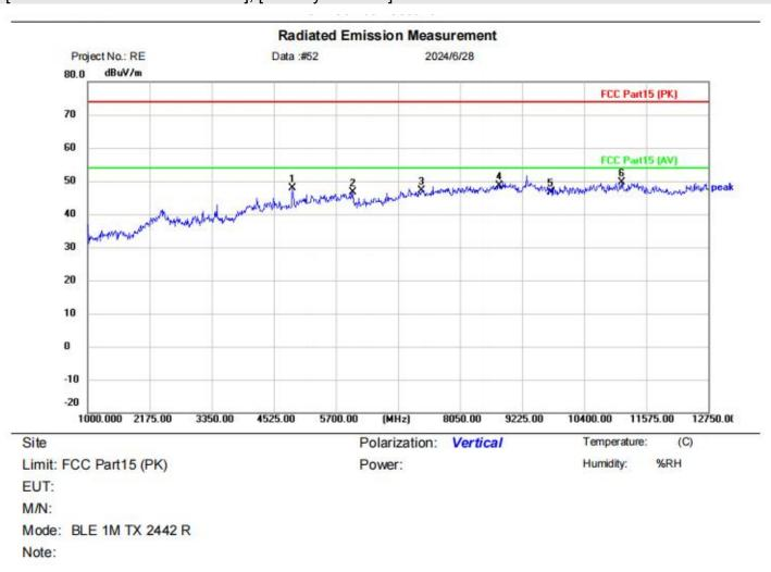
[Test mode: TX middle channel]; [Polarity: Vertical]
