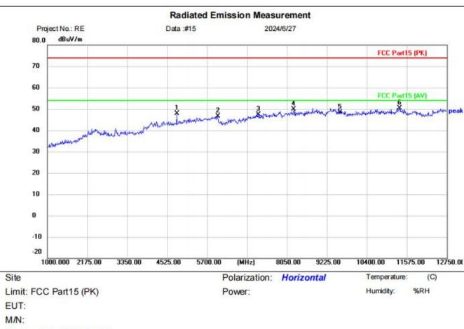
[Test mode: TX low channel]; [Polarity: Horizontal]
