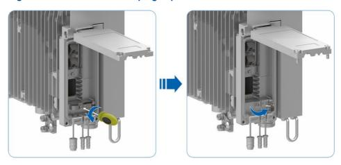
8. Insert the conductor plug into the power port inside the maintenance window, see Figure 5-12. Push the plug forward unit you hear the sound of "click". If you shake the plug shell but it does not loosen or fall down (you are not allowed to pull the plug's pull-tab at this time), it indicates that the plug is installed securely and locked closely.
