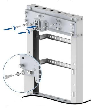
2. Fix the RRU support to the back of the RRU with four M6 screws with a torque of 8 N•m, see Figure 4-37.
