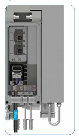
9. Use the crimping clip to crimp the naked part of the shielding layer, secure the power cable at the original waterproof plug, and ensure that the naked part has a close contact with the crimping clip.
