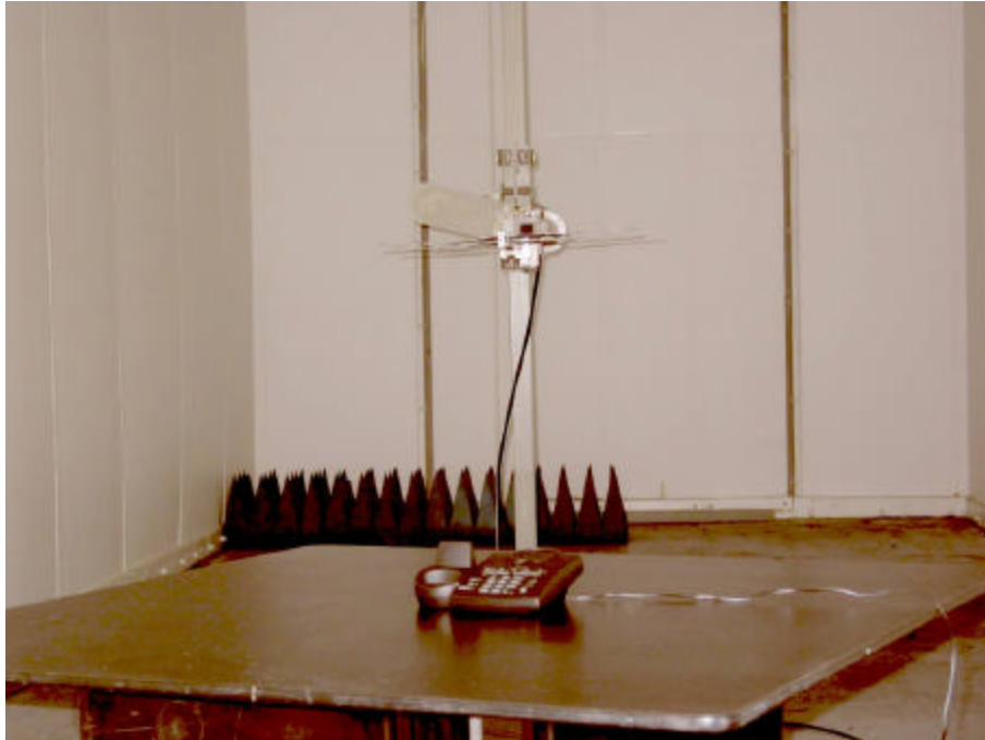
Uniden – Base Unit Testing for Radiated Emissions from Transmitter Frequency Range: 200 MHz – 1 GHz
