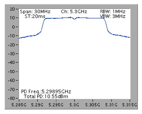
Power Density Plot on Configuration IEEE 802.11a / Chain 3 / 5580 MHz
