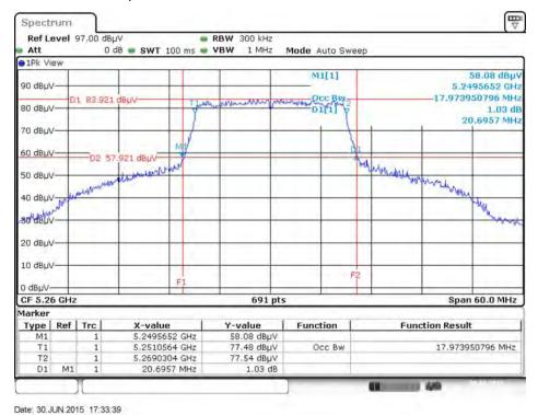
26dB Bandwidth and 99% Occupied Bandwidth Plot on Configuration IEEE 802.11ac MCS0/Nss1 VHT20 / Chain 3 + Chain 4 + Chain 5 / 5300 MHz
