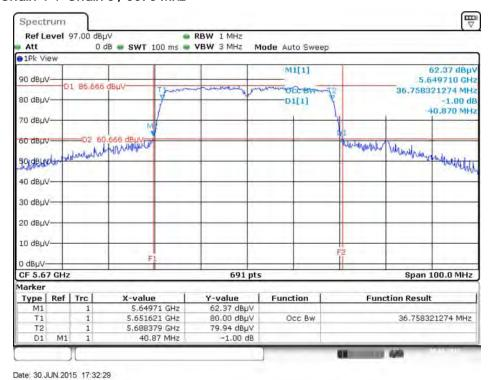
26dB Bandwidth and 99% Occupied Bandwidth Plot on Configuration IEEE 802.11ac MCS0/Nss1 VHT80 / Chain 3 + Chain 4 + Chain 5 / 5290 MHz
