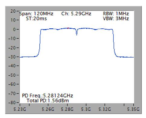
Power Density Plot on Configuration IEEE 802.11ac MCS0/Nss1 VHT80 / Chain 3 + Chain 4 + Chain 5 / 5530 MHz
