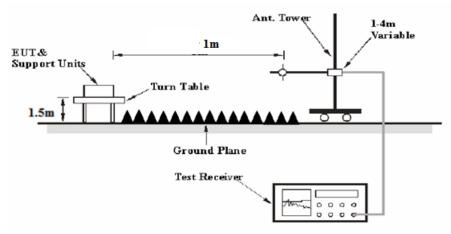
The radiated emission below 1GHz tests were performed in the 3 meters chamber test site A, above 1GHz tests were performed in the 3 meters chamber test site B, using the setup accordance with the ANSI C63.10-2013. The specification used was the FCC 15.209, and FCC 15.407.
