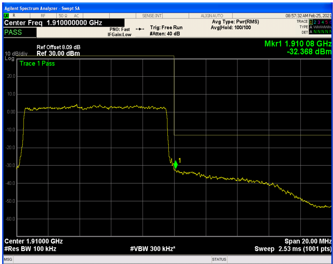
Band2 QAM16 BW=10MHz Channel=19150 RB Size=1 Position=#Max
