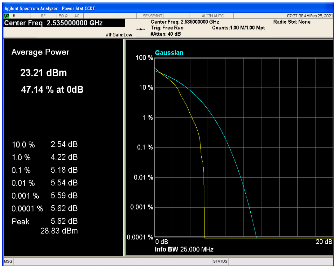
Band7 QAM16 BW=10MHz Channel=21100 RB Size=1 Position=#0
