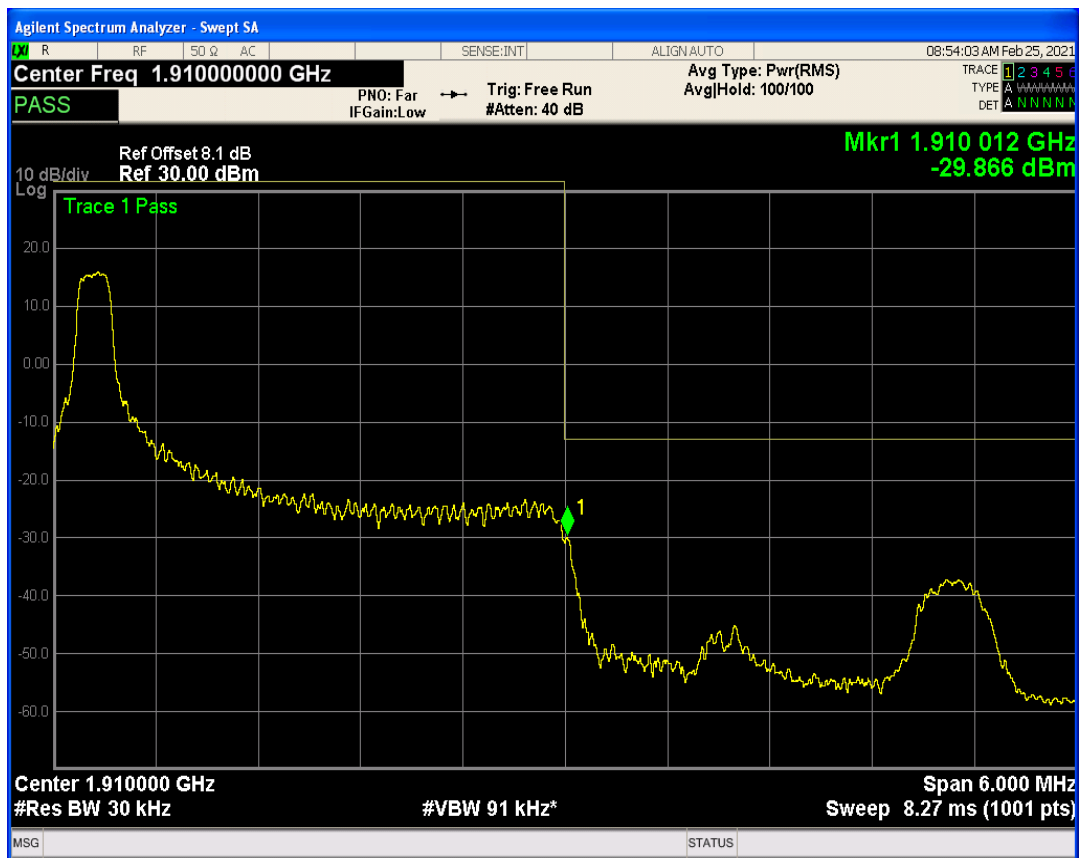
Band2 QPSK BW=3MHz Channel=19185 RB Size=1 Position=#Max
