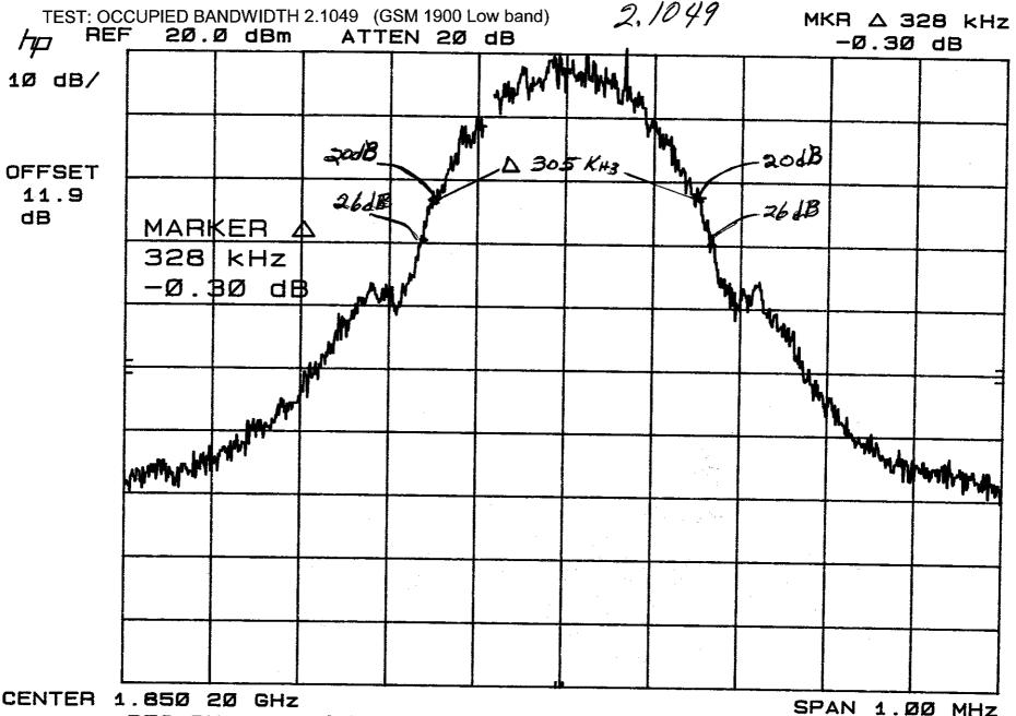
CENTER 1.850 20 GHz RES BW 3 kHz (i) VBW 3 kHz
