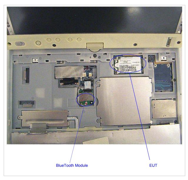
WLAN MODULE AND BLUETOOTH MODULE
