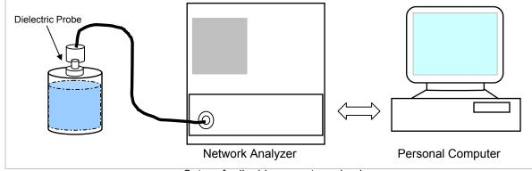
Set-up for liquid parameters check
