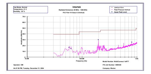
Intertek Testing Services Radiated Emissions 30 MHz - 1000 MHz FCC Part 15 Class A (QP-Vertical)
