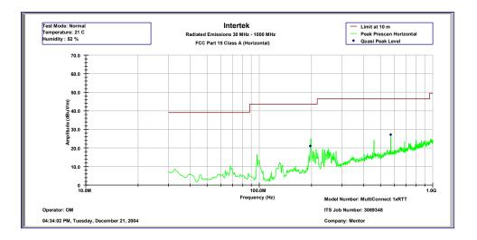
Intertek Testing Services Radiated Emissions 30 MHz - 1000 MHz FCC Part 15 Class A (QP-Horizontal)
