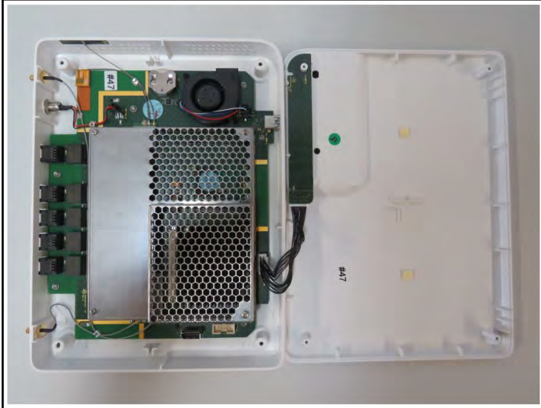
EUT PCB FRONT (with shielding)
