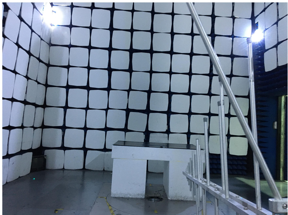
Radiation Emission Test Setup (30MHz to 1GHz)
