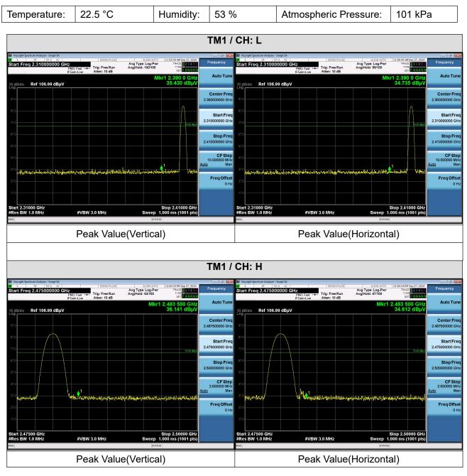
Note: When the PK measure result value is less than the AVG limit value, the AV measure result values test not applicable.
