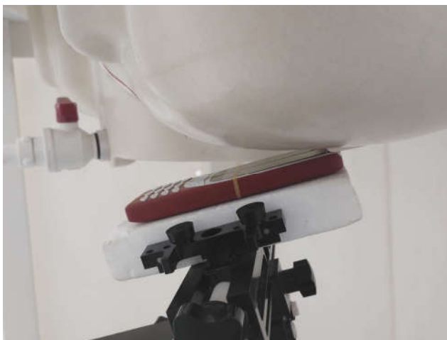
Left Tilted, Test Separation 0 mm
