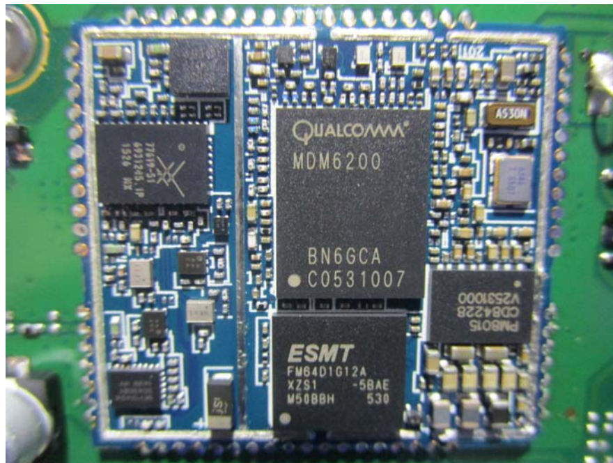
EUT- WCDMA Module Uncover View
