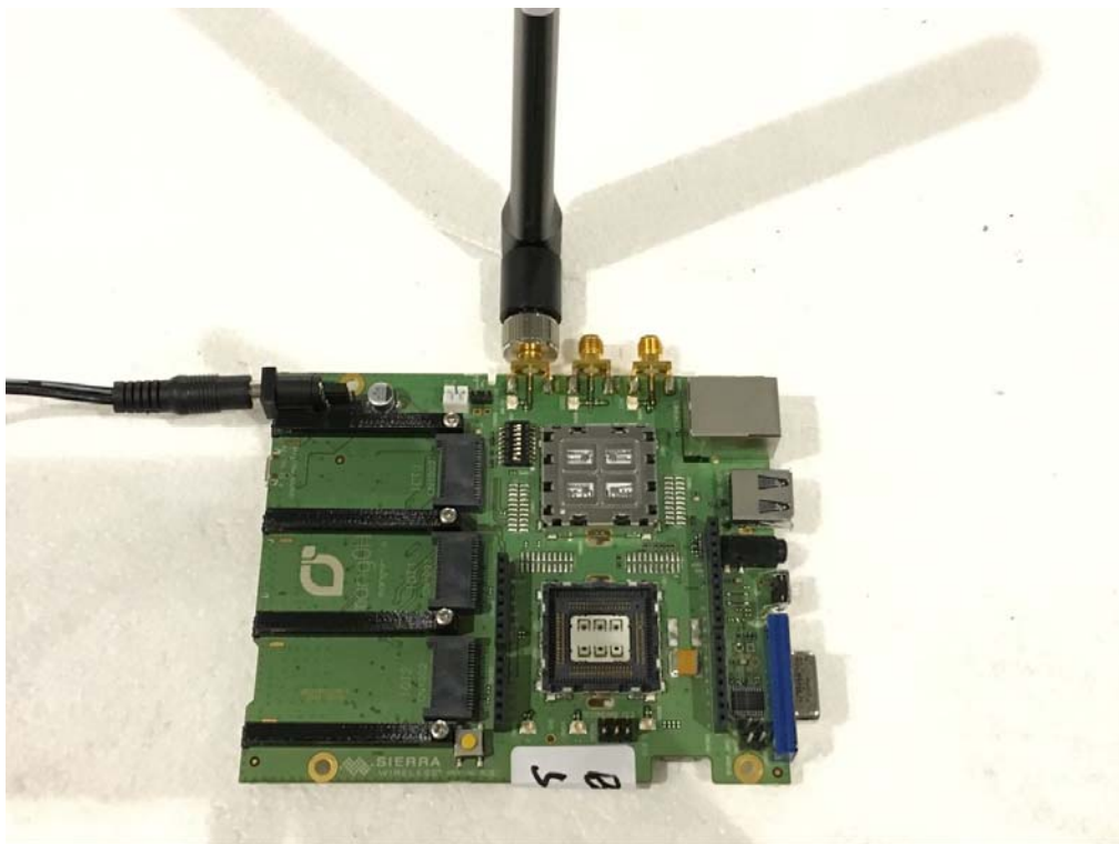
Pic.2 Radiated test set-up 1
