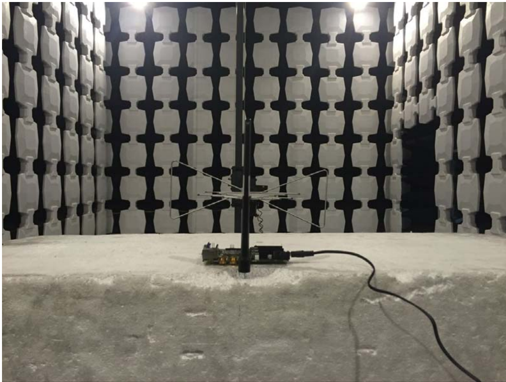
Pic.3 Radiated test set-up 2
