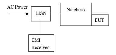
The EUT are connected to the main power through a line impedance stabilization network (LISN). This provides a 50 ohm/50uH coupling impedance for the measuring equipment. The peripheral devices are also connected to the main power through a LISN that provides a 500hm/50uH coupling impedance with 500hm termination.
