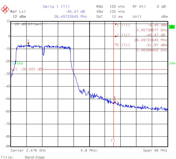
Test Mode: 802.11g mode Tx at channel 11
