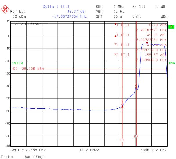
Test Mode: 802.11g mode Tx at channel 1
