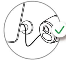
For optimal waterproofing, ensure the cable's low point hangs below the charging ports of the solar panel and device, utilizing gravity to direct water away from the charging area.
