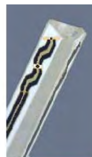
Figure E.2.2 Probe Thick-Film Technique
