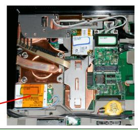
The certification label is stuck on the topside of the applying transmitter device, and the FCC ID is visible when the keyboard assembly is removed.
