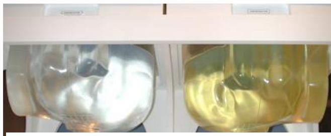
Figure 7.1 Left and Right SAM Phantom shells
