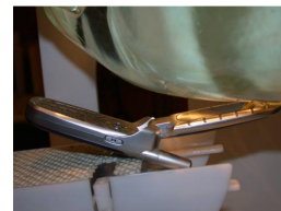
Figure A.4 Left Head SAR Test Setup -- Ear / 15° Tilt Position --
