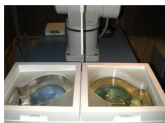
Figure 5.2 Head Simulated Tissue
