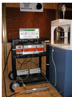
Figure A.0 Dipole Validation Test Setup
