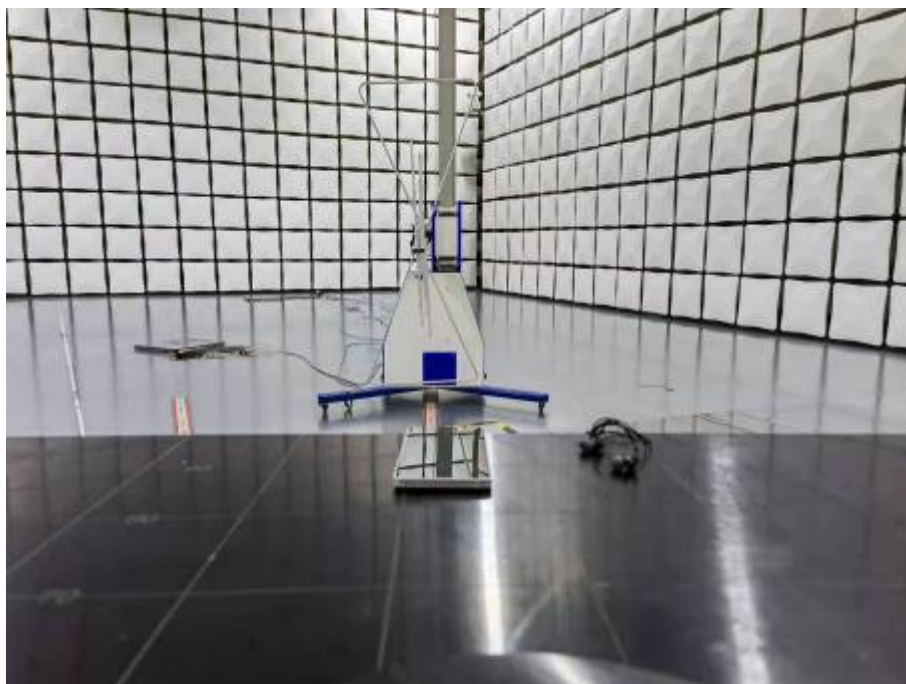
Radiated Emissions Test Setup (30-1000MHz)
