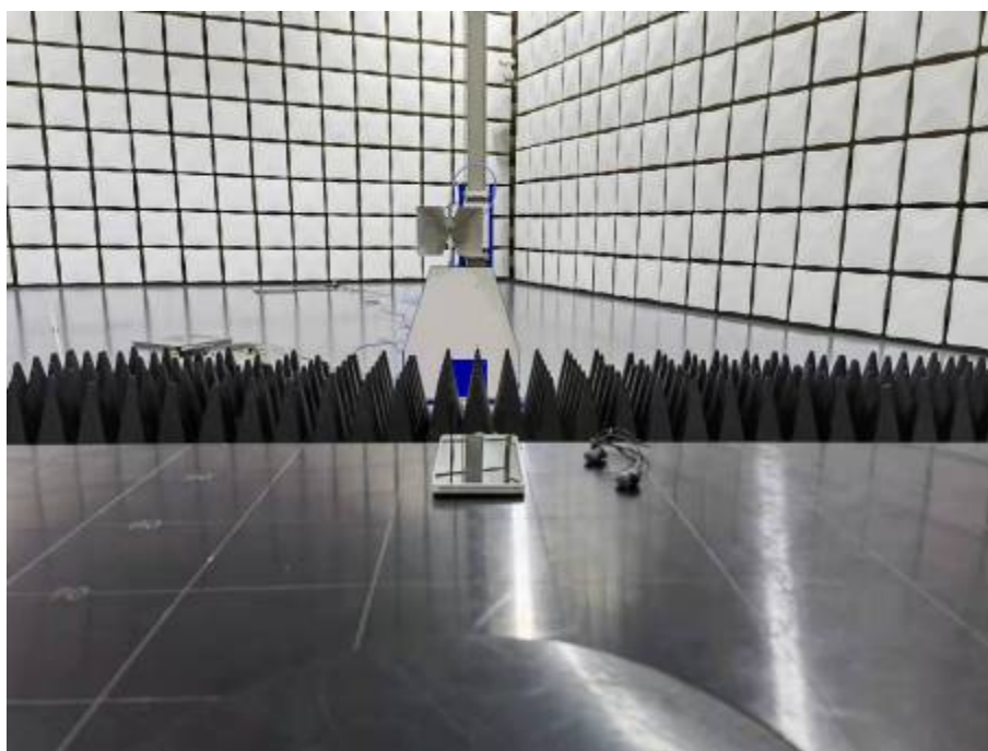
Radiated Emissions Test Setup (above 1GHz)
