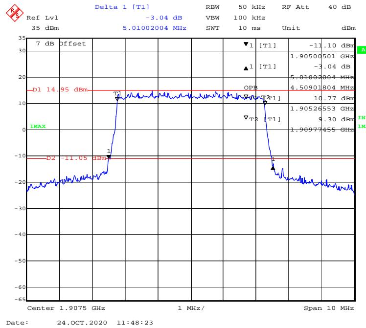
**16-QAM (10 MHz) - 99% Occupied & 26 dB Emissions Bandwidth, High channel**
