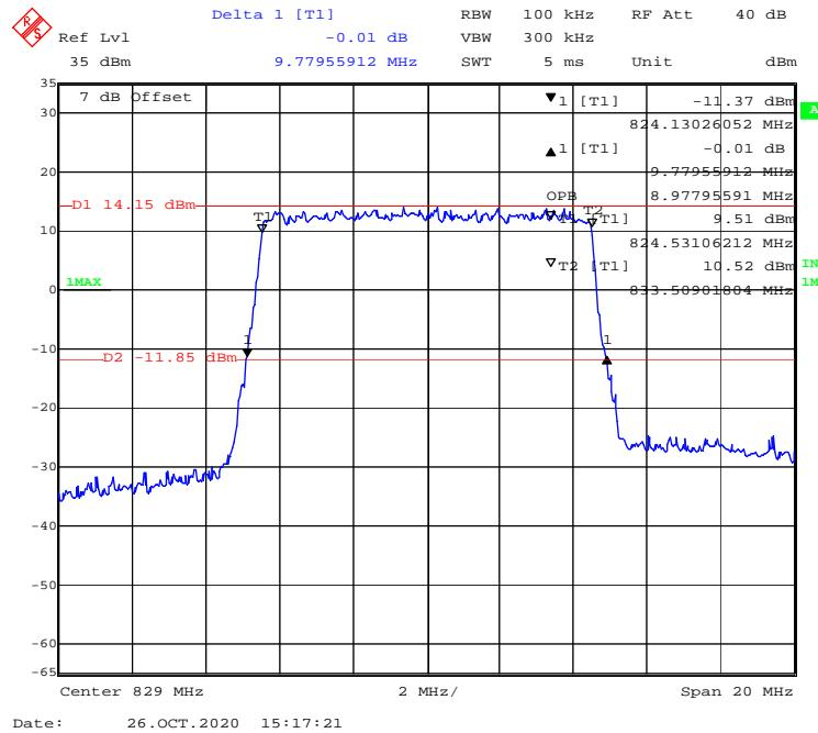
**QPSK (1.4 MHz) - 99% Occupied & 26 dB Emissions Bandwidth, Middle channel**
