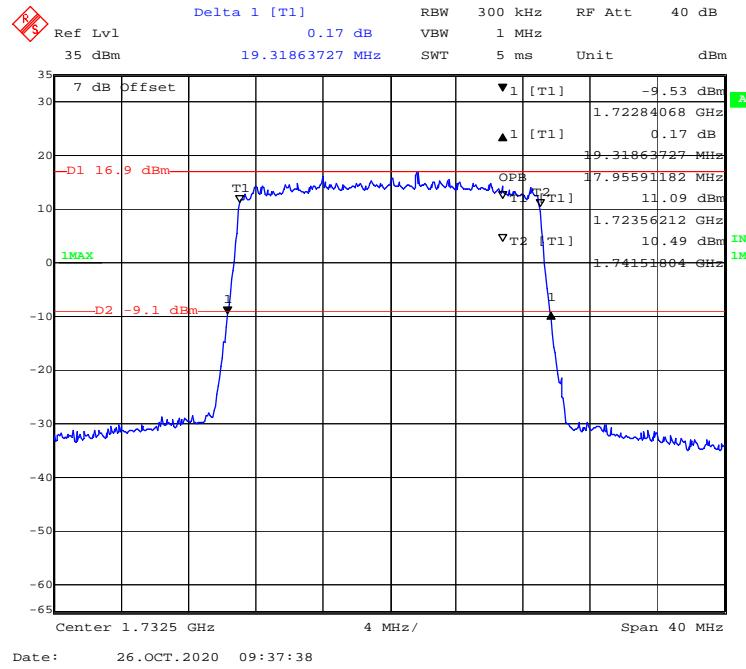
**QPSK (1.4 MHz) - 99% Occupied & 26 dB Emissions Bandwidth, High channel**
