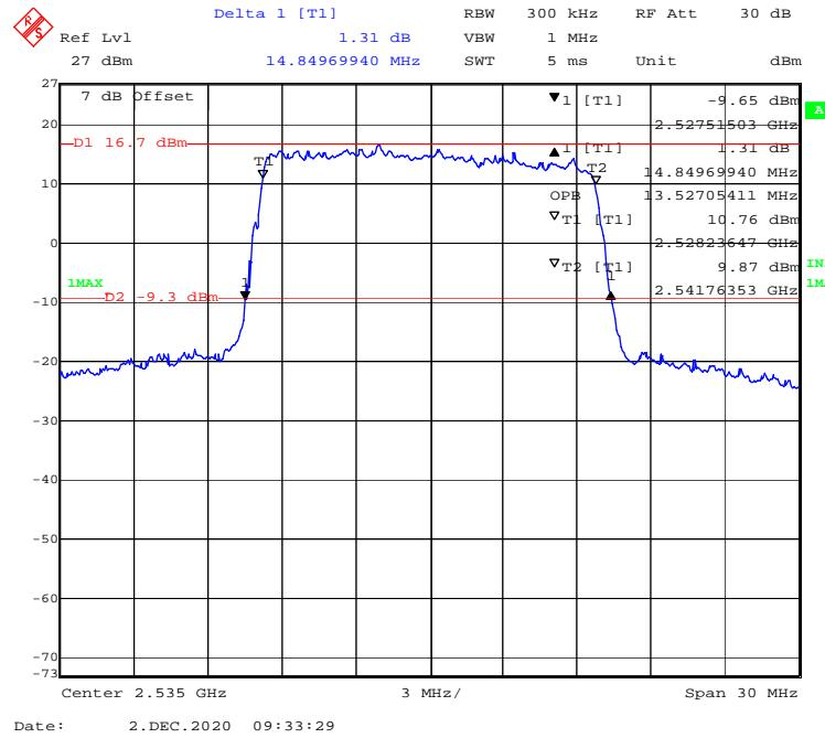
**16-QAM (20 MHz) - 99% Occupied & 26 dB Emissions Bandwidth, Middle channel**
