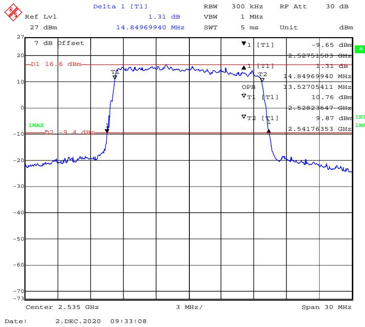
**QPSK (20 MHz) - 99% Occupied & 26 dB Emissions Bandwidth, Middle channel**
