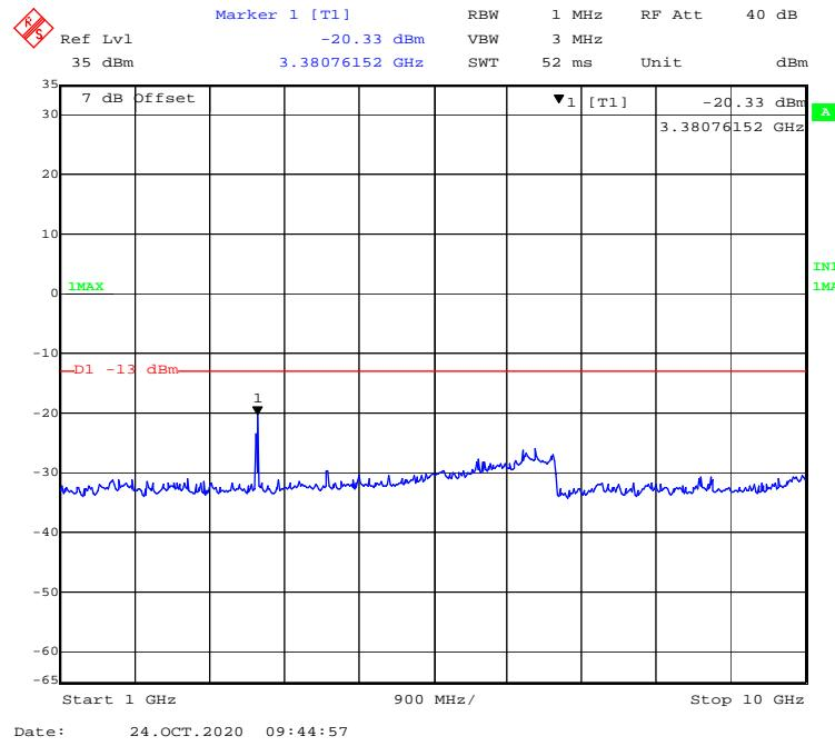
**PCS 1900 Band:****30 MHz – 1GHz(GSM Mode) , Low channel**
