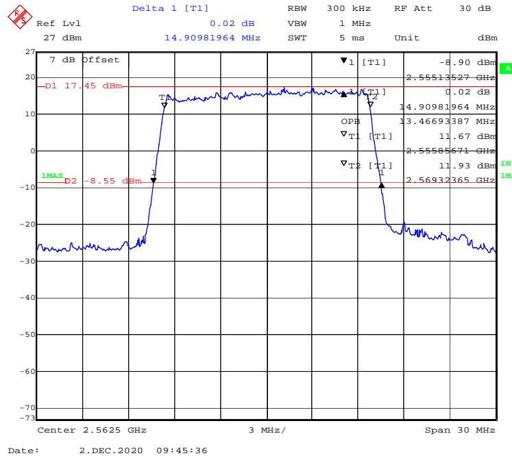
**16-QAM (20 MHz) - 99% Occupied & 26 dB Emissions Bandwidth, High channel**
