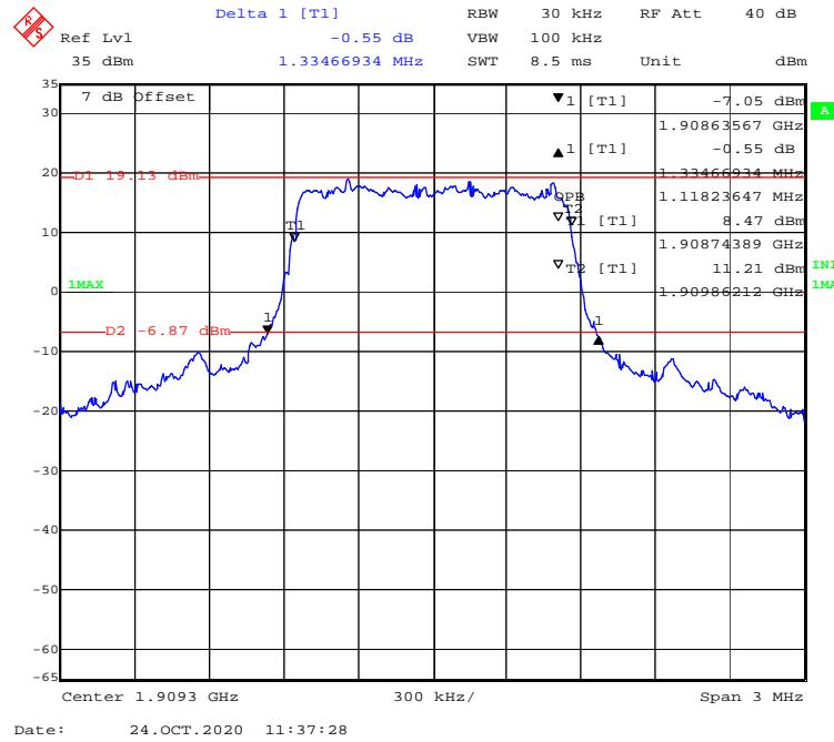
**QPSK (3 MHz) - 99% Occupied & 26 dB Emissions Bandwidth, High channel**
