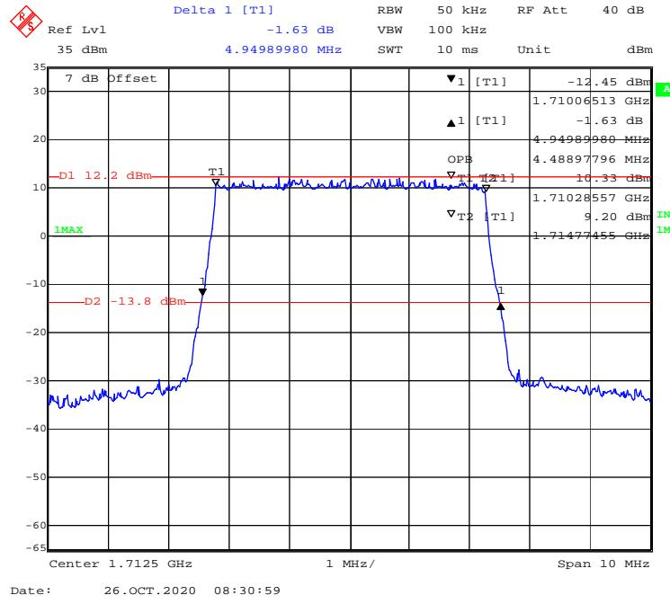
**16-QAM (10 MHz) - 99% Occupied & 26 dB Emissions Bandwidth, Low channel**
