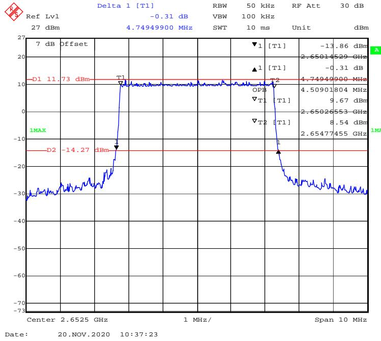
**QPSK (10 MHz) - 99% Occupied & 26 dB Emissions Bandwidth, High channel**
