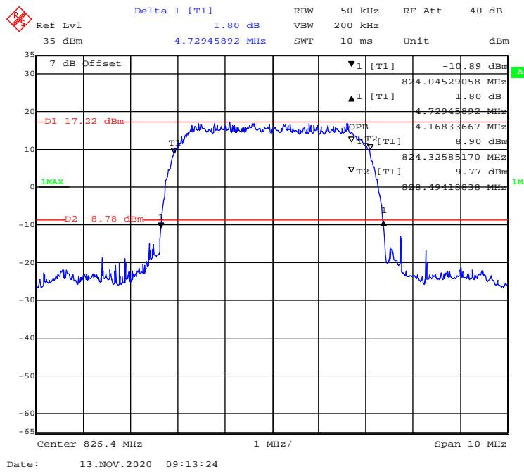
**99% Occupied & 26 dB Emissions Bandwidth for WCDMA (HSUPA) Middle channel**
