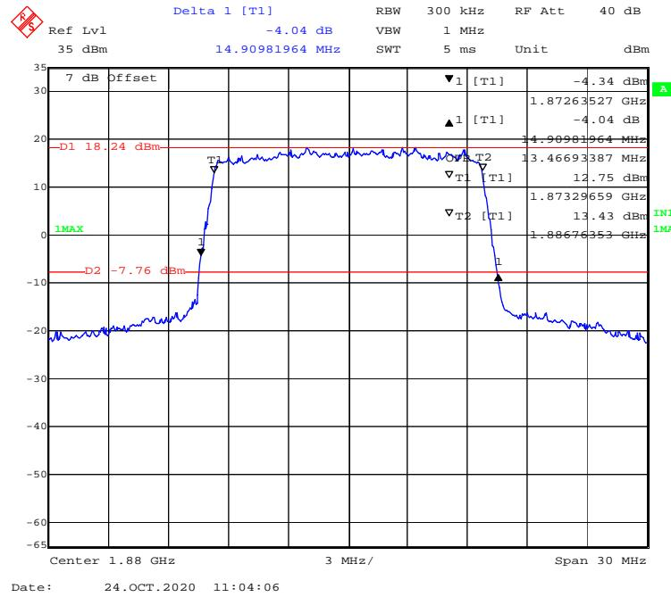
**QPSK (20 MHz) - 99% Occupied & 26 dB Emissions Bandwidth, Middle channel**
