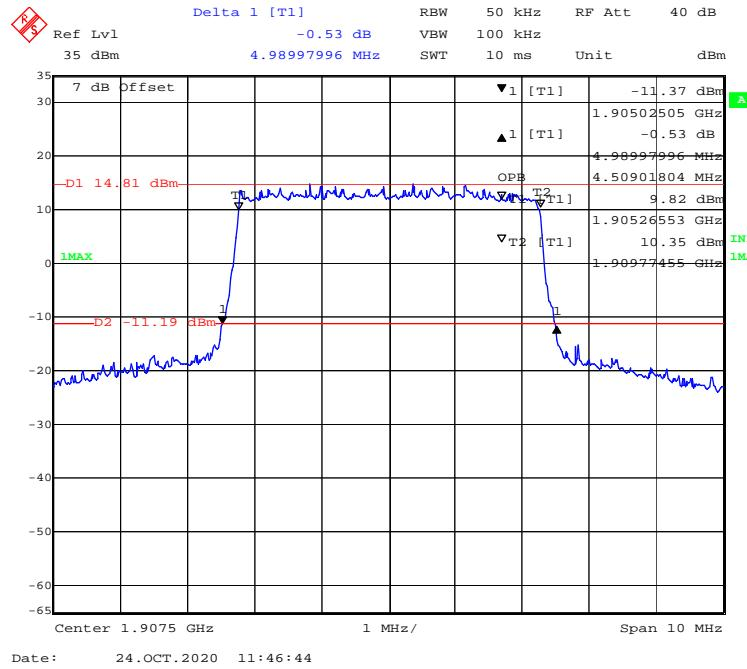
**QPSK (10MHz) - 99% Occupied & 26 dB Emissions Bandwidth, High channel**
