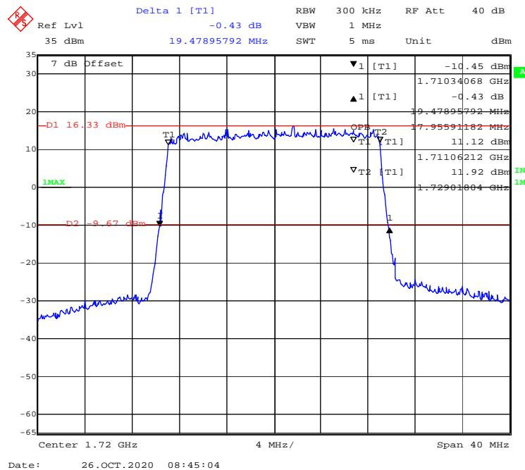
**QPSK (1.4 MHz) - 99% Occupied & 26 dB Emissions Bandwidth, Middle channel**
