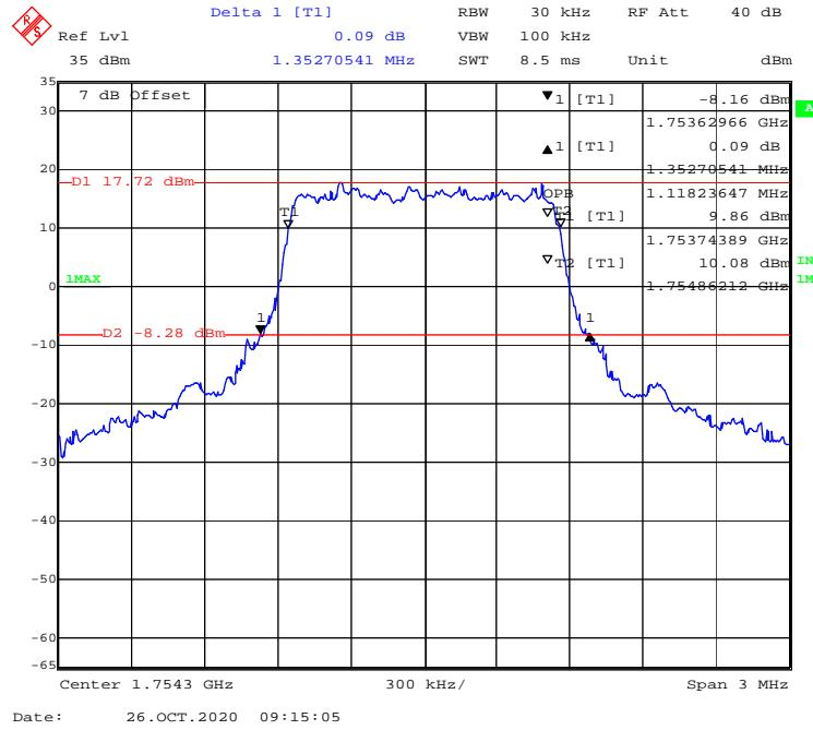
**16-QAM (3 MHz) - 99% Occupied & 26 dB Emissions Bandwidth, High channel**
