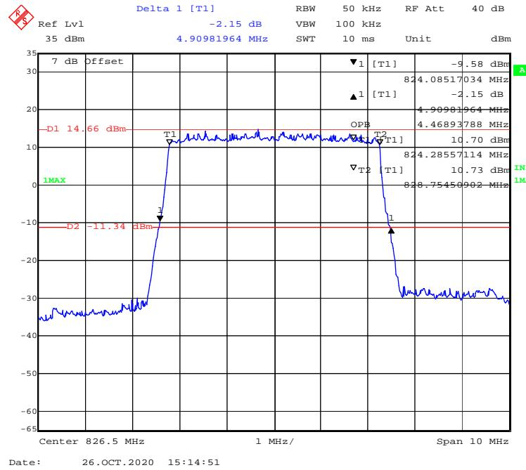
**16-QAM (10.0 MHz) - 99% Occupied & 26 dB Emissions Bandwidth, Low channel**
