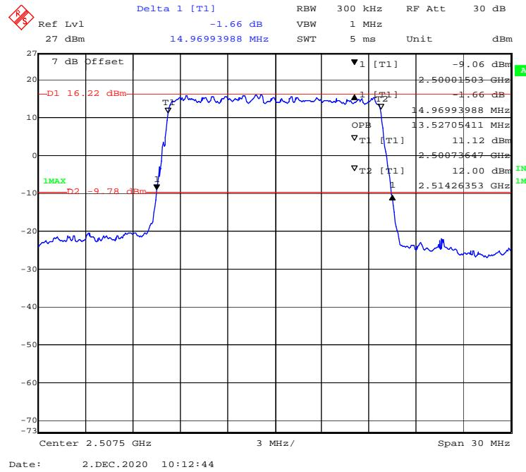
**16-QAM (20 MHz) - 99% Occupied & 26 dB Emissions Bandwidth, Low channel**
