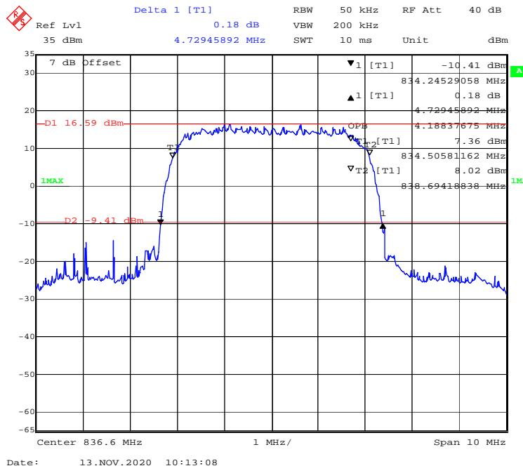
**99% Occupied & 26 dB Emissions Bandwidth for WCDMA (HSUPA) High channel**
