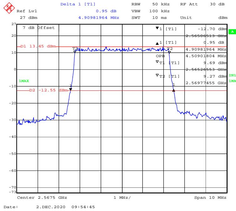
**QPSK (10 MHz) - 99% Occupied & 26 dB Emissions Bandwidth, High channel**
