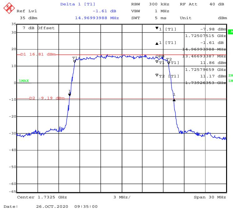
**16-QAM (20 MHz) - 99% Occupied & 26 dB Emissions Bandwidth, Middle channel**
