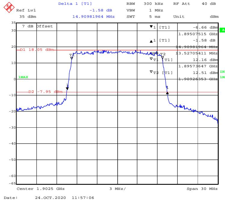
**QPSK (20 MHz) - 99% Occupied & 26 dB Emissions Bandwidth, High channel**
