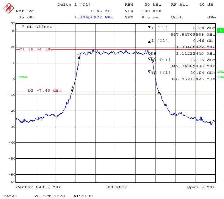
**QPSK (3.0 MHz) - 99% Occupied & 26 dB Emissions Bandwidth, High channel**
