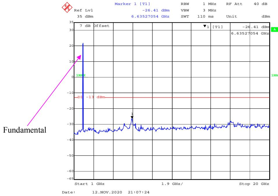
**30 MHz – 1GHz WCDMA (HSPA+) Mode , Middle channel**
