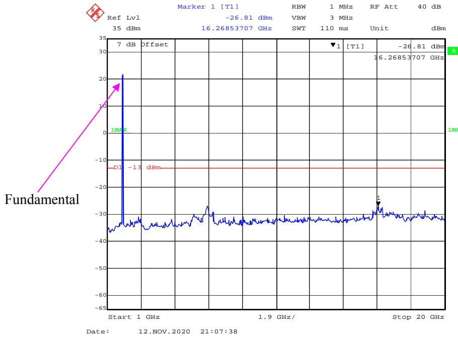
**30 MHz – 1GHz WCDMA (Rel 99) Mode , High channel**
