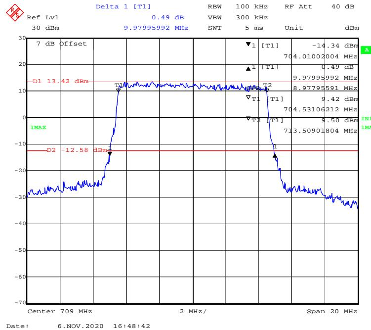
**QPSK (5 MHz) - 99% Occupied & 26 dB Emissions Bandwidth, Middle channel**
