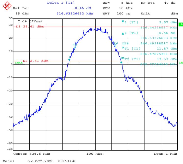
**99% Occupied & 26 dB Emissions Bandwidth for GPRS (GMSK) High channel**
