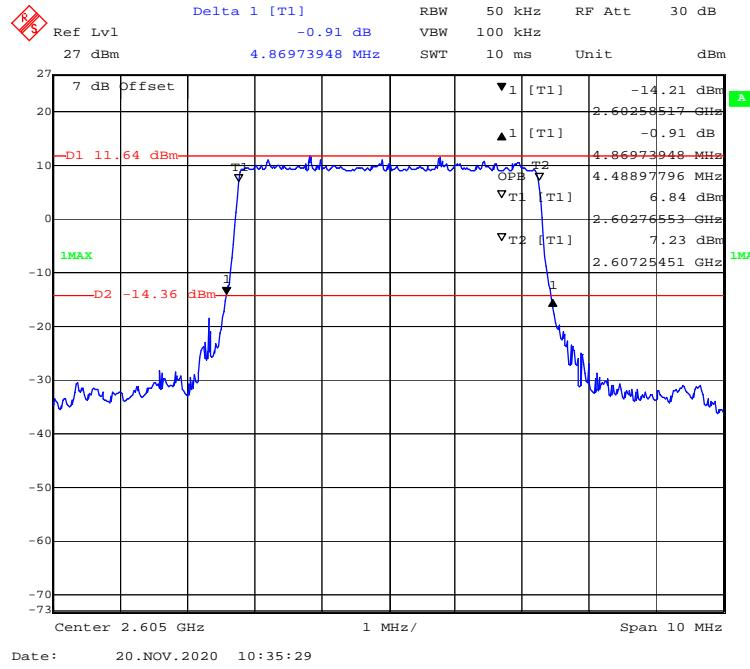
**QPSK (10 MHz) - 99% Occupied & 26 dB Emissions Bandwidth, Middle channel**
