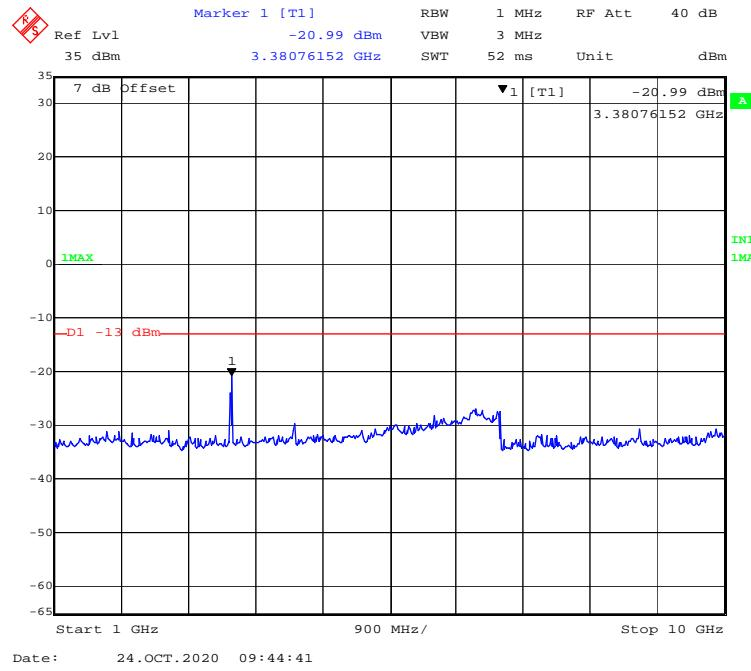
**30 MHz – 1GHz WCDMA (HSPA+) Mode, High channel**
