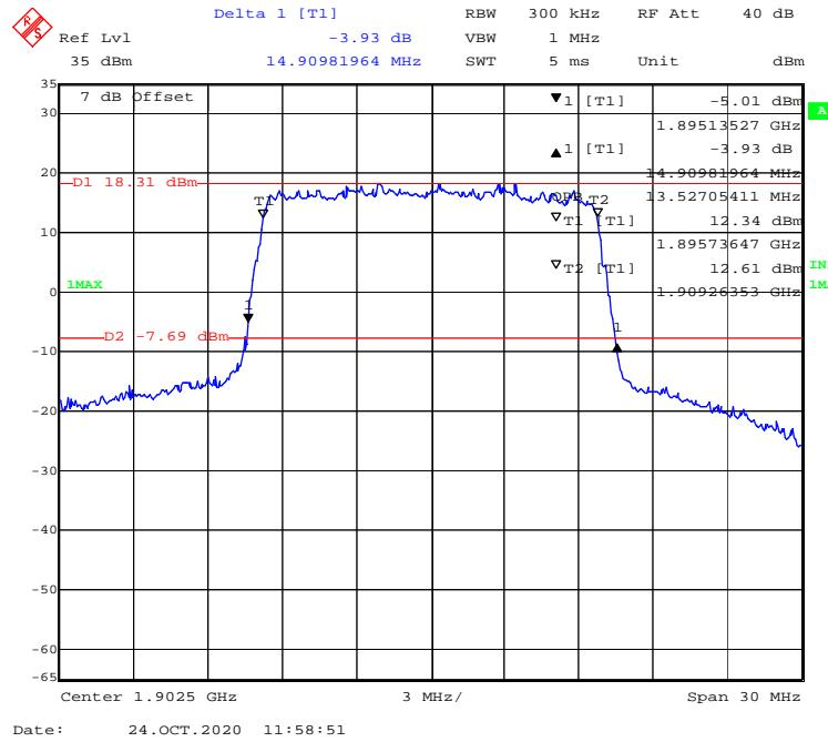
**16-QAM (20 MHz) - 99% Occupied & 26 dB Emissions Bandwidth, High channel**
