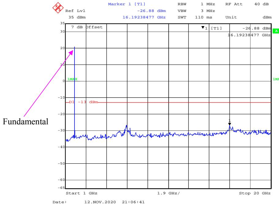
**30 MHz – 1GHz WCDMA (Rel 99) Mode , Middle channel**
