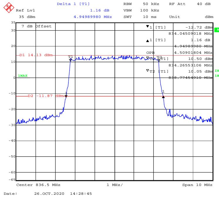
**QPSK (10.0 MHz) - 99% Occupied & 26 dB Emissions Bandwidth, Middle channel**
