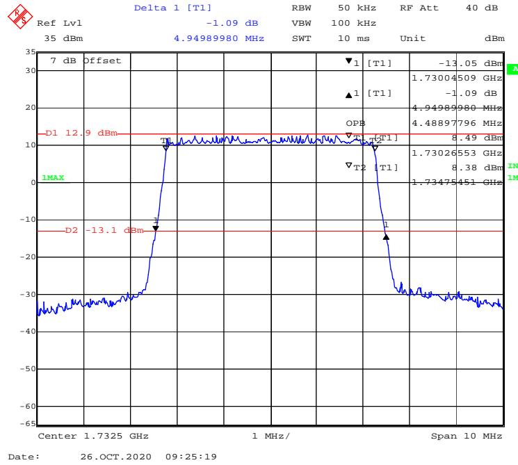
**QPSK (10 MHz) - 99% Occupied & 26 dB Emissions Bandwidth, Middle channel**
