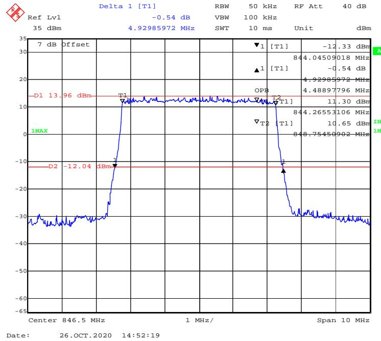
**16-QAM (10.0 MHz) - 99% Occupied & 26 dB Emissions Bandwidth, High channel**
