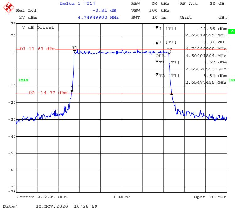
**16-QAM (10 MHz) - 99% Occupied & 26 dB Emissions Bandwidth, High channel**
