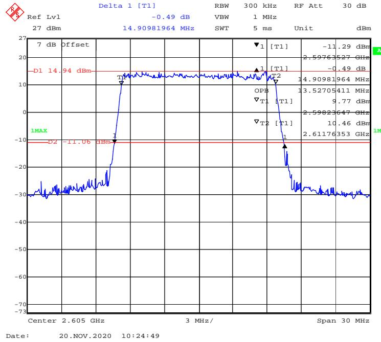
**QPSK (20 MHz) - 99% Occupied & 26 dB Emissions Bandwidth, Middle channel**
