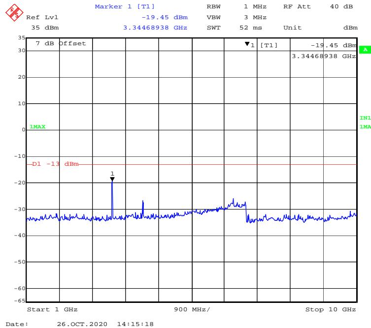
**30 MHz - 1 GHz (16QAM, 1.4 MHz, Middle Channel)**
