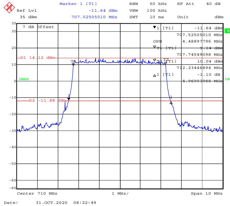
**16-QAM (10 MHz) - 99% Occupied & 26 dB Emissions Bandwidth, Middle channel**
