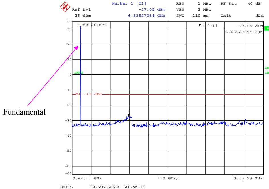
**30 MHz – 1GHz(GPRS Mode) , Low channel**
