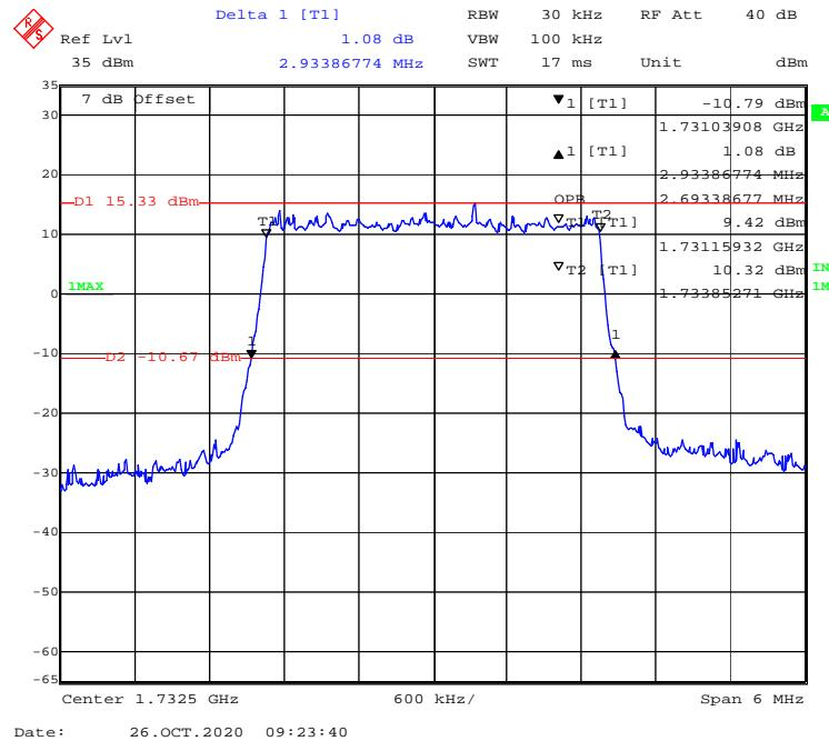
**16-QAM (5 MHz) - 99% Occupied & 26 dB Emissions Bandwidth, Middle channel**
