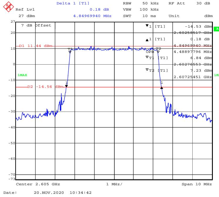
**16-QAM (10 MHz) - 99% Occupied & 26 dB Emissions Bandwidth, Middle channel**
