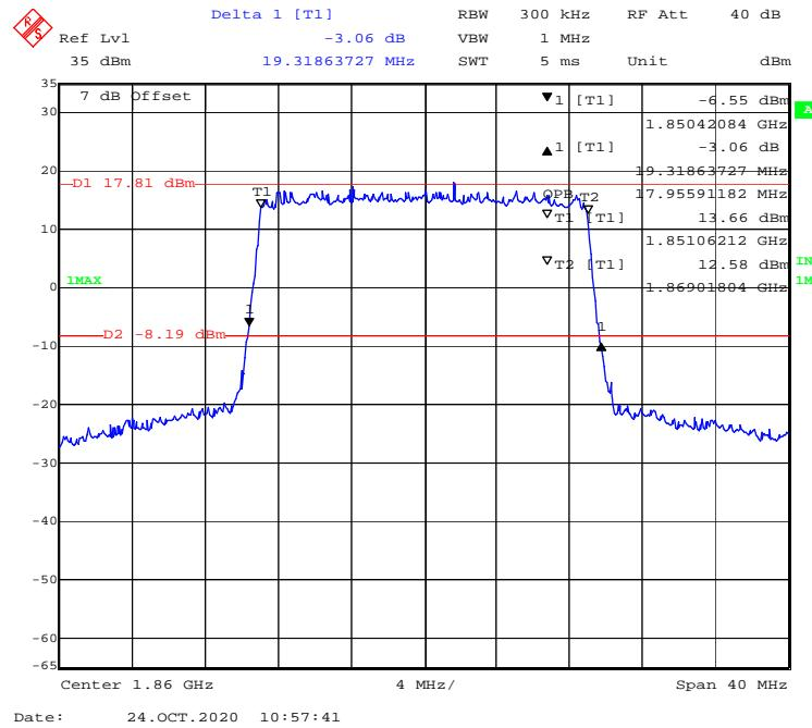
**QPSK (1.4 MHz) - 99% Occupied & 26 dB Emissions Bandwidth, Middle channel**
