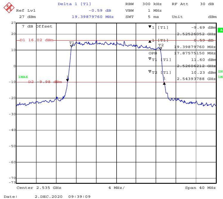
**16-QAM (5 MHz) - 99% Occupied & 26 dB Emissions Bandwidth, High channel**
