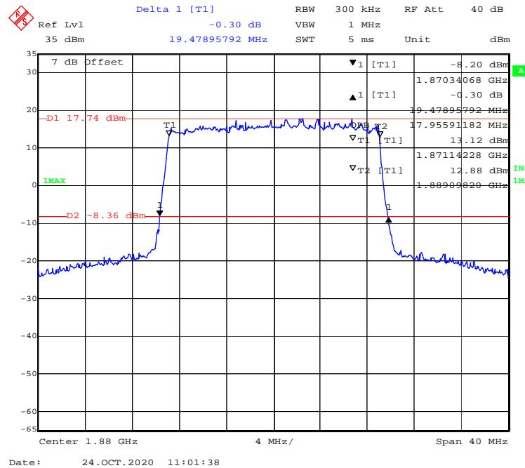
**16-QAM (1.4 MHz) - 99% Occupied & 26 dB Emissions Bandwidth, High channel**
