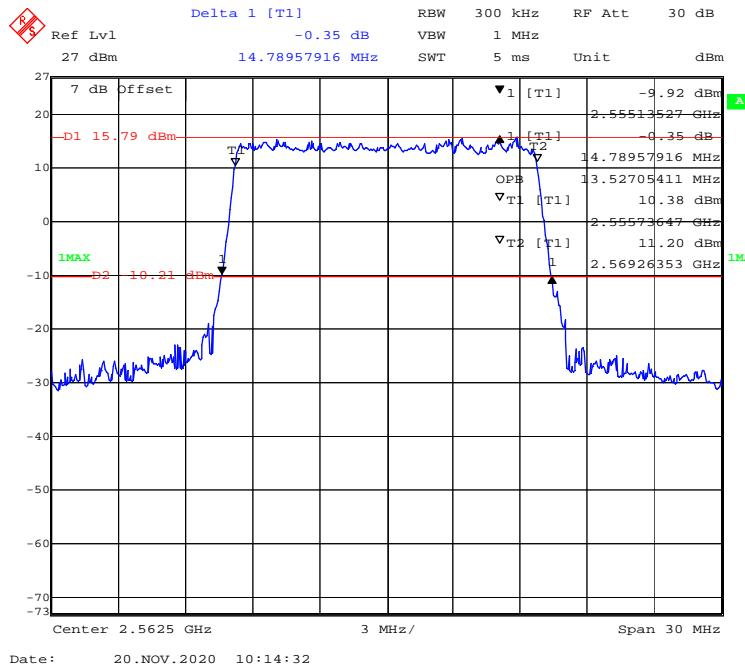
**QPSK (20 MHz) - 99% Occupied & 26 dB Emissions Bandwidth, Low channel**
