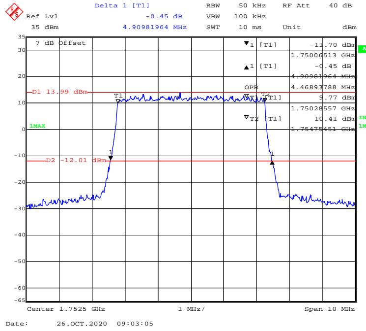
**QPSK (10 MHz) - 99% Occupied & 26 dB Emissions Bandwidth, High channel**
