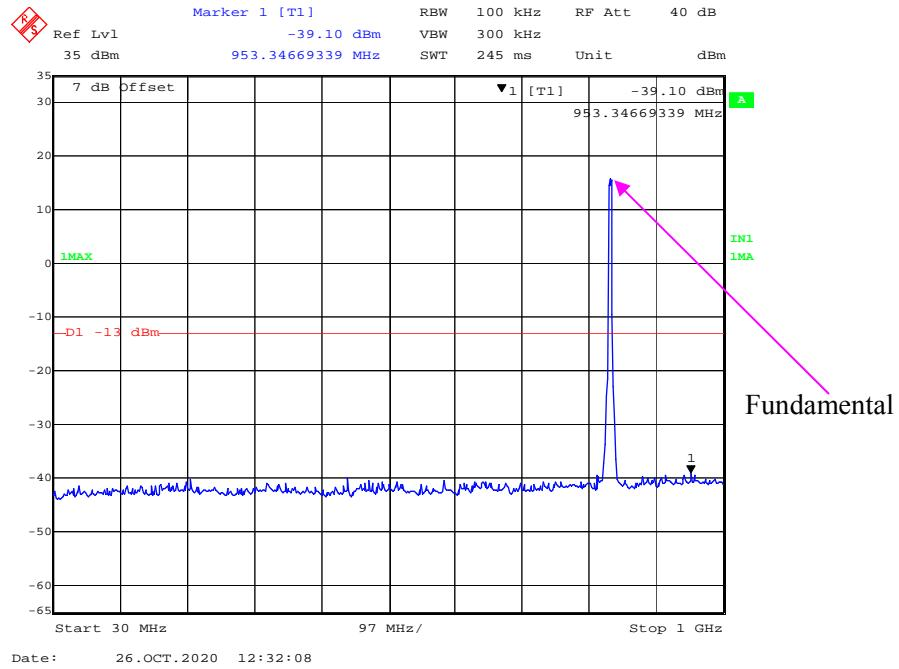
**1 GHz – 10 GHz (16QAM, 5.0MHz, Middle Channel)**
