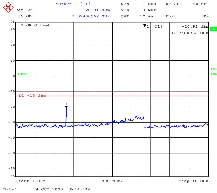
**30 MHz – 1GHz WCDMA (HSUPA) Mode, Low channel**
