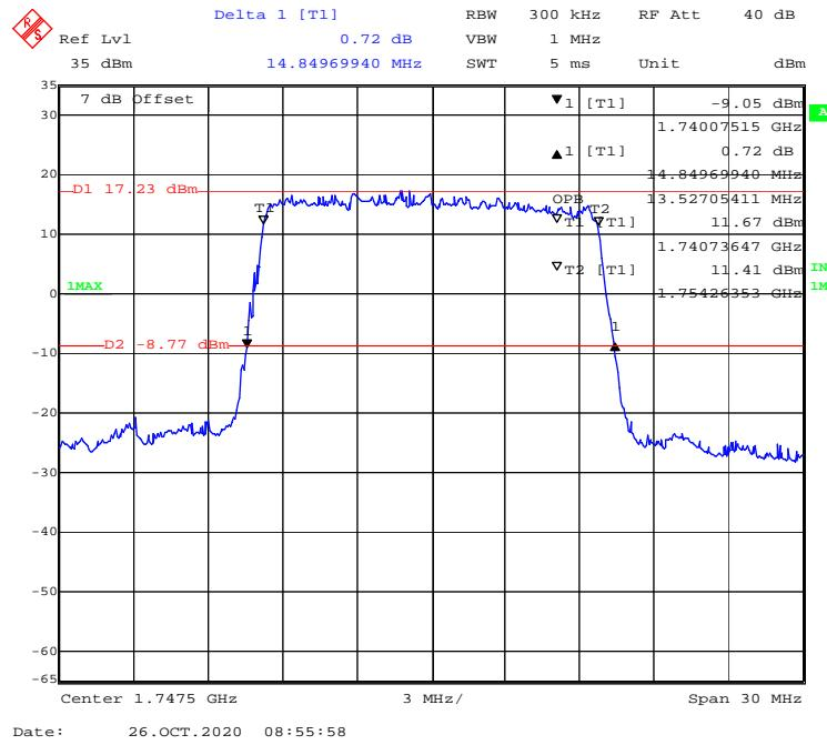
**16-QAM (20 MHz) - 99% Occupied & 26 dB Emissions Bandwidth, High channel**
