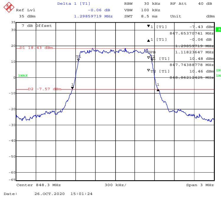
**16-QAM (3.0 MHz) - 99% Occupied & 26 dB Emissions Bandwidth, High channel**
