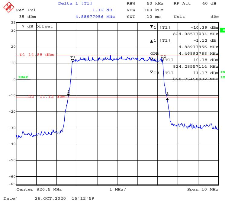
**QPSK (10.0 MHz) - 99% Occupied & 26 dB Emissions Bandwidth, Low channel**
