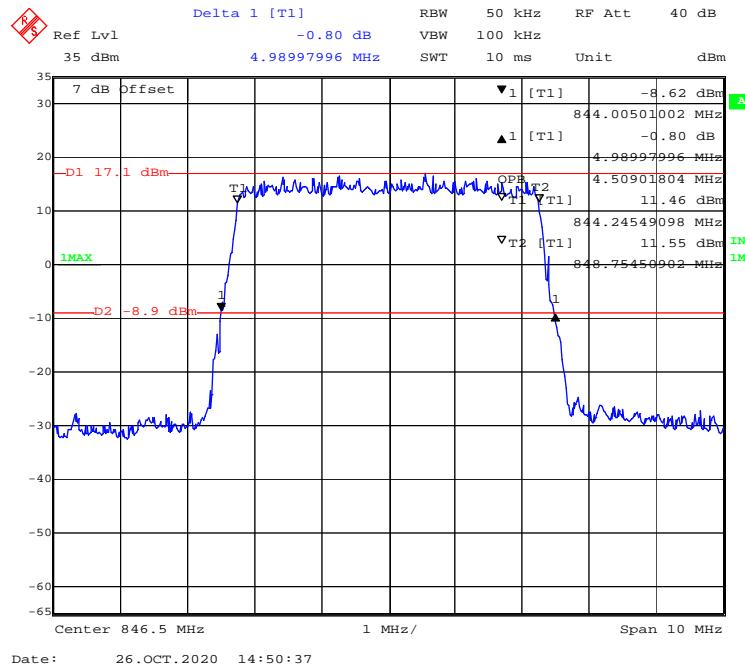
**QPSK (10.0 MHz) - 99% Occupied & 26 dB Emissions Bandwidth, High channel**
