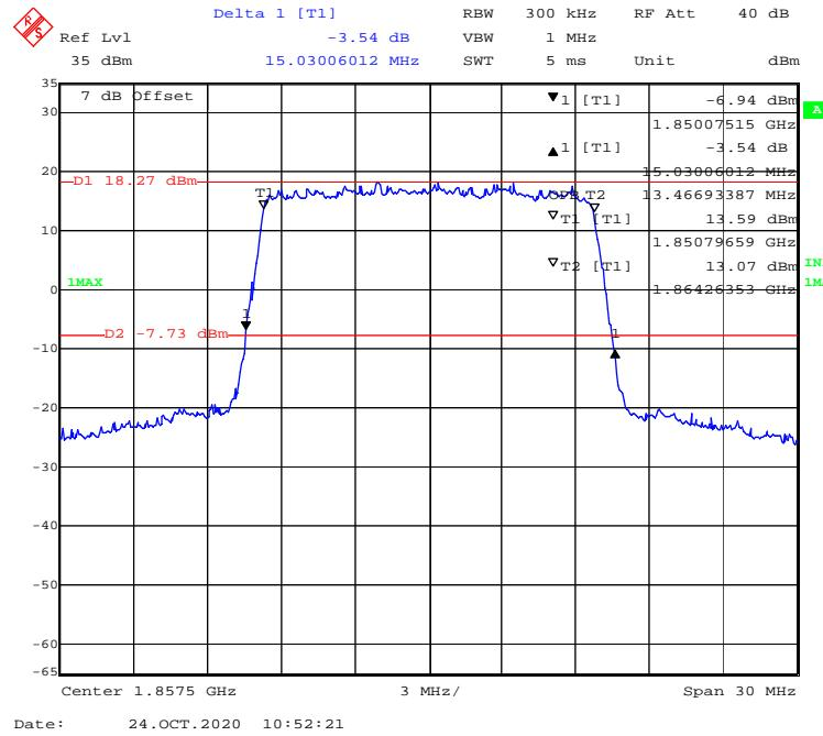
**16-QAM (20 MHz) - 99% Occupied & 26 dB Emissions Bandwidth, Low channel**
