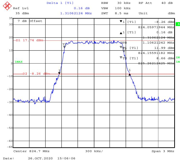
**16-QAM (3.0 MHz) - 99% Occupied & 26 dB Emissions Bandwidth, Low channel**
