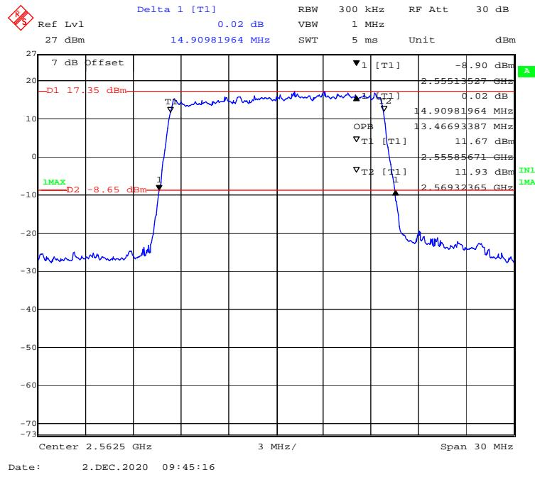
**QPSK (20 MHz) - 99% Occupied & 26 dB Emissions Bandwidth, High channel**
