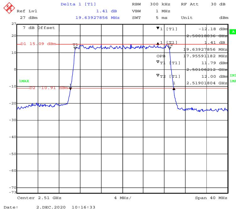
**QPSK (5 MHz) - 99% Occupied & 26 dB Emissions Bandwidth, Middle channel**
