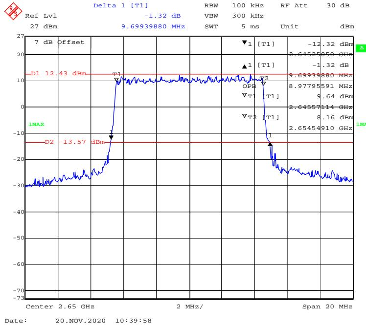
**16-QAM (15 MHz) - 99% Occupied & 26 dB Emissions Bandwidth, High channel**
