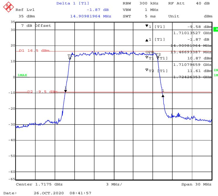
**QPSK (20 MHz) - 99% Occupied & 26 dB Emissions Bandwidth, Low channel**
