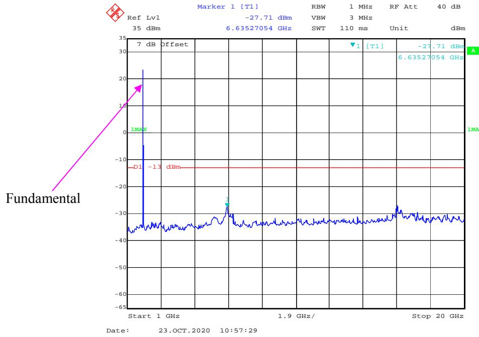
**WCDMA Band II:****30 MHz – 1GHz WCDMA (Rel 99) Mode , Low channel**
