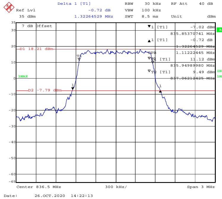
**16-QAM (3.0 MHz) - 99% Occupied & 26 dB Emissions Bandwidth, Middle channel**
