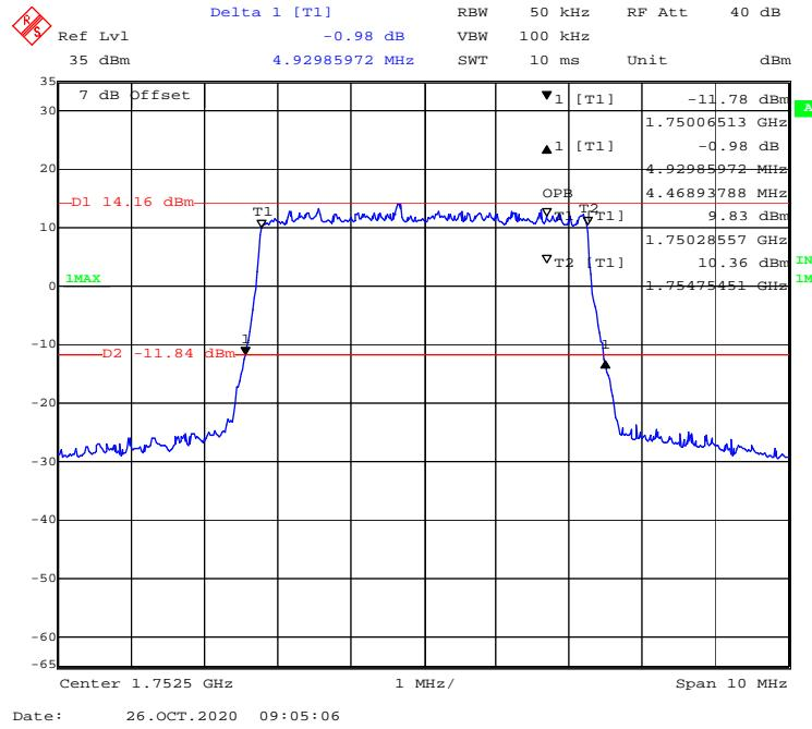
**16-QAM (10 MHz) - 99% Occupied & 26 dB Emissions Bandwidth, High channel**
