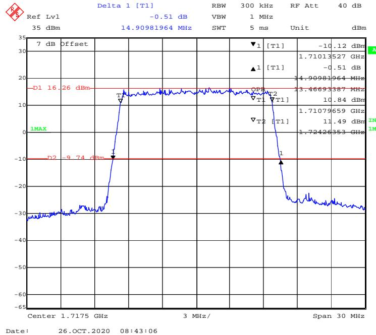
**16-QAM (20 MHz) - 99% Occupied & 26 dB Emissions Bandwidth, Low channel**
