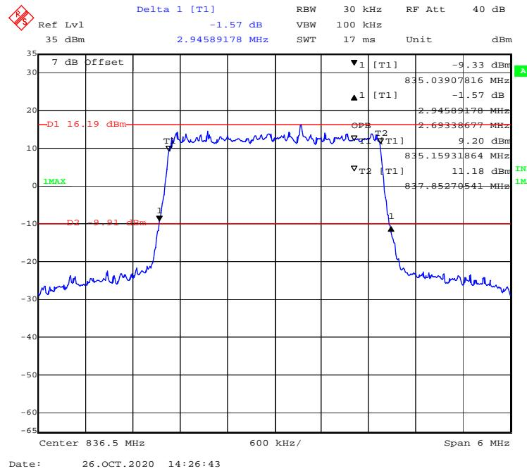
**16-QAM (5.0 MHz) - 99% Occupied & 26 dB Emissions Bandwidth, Middle channel**
