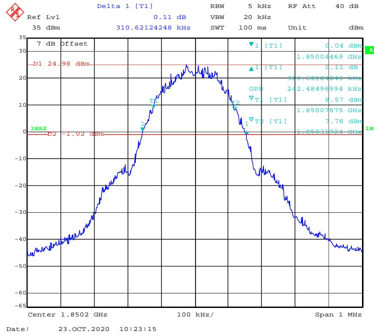
**99% Occupied & 26 dB Emissions Bandwidth for GSM (GMSK) Middle channel**
