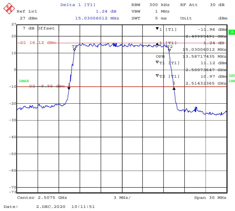
**QPSK (20 MHz) - 99% Occupied & 26 dB Emissions Bandwidth, Low channel**
