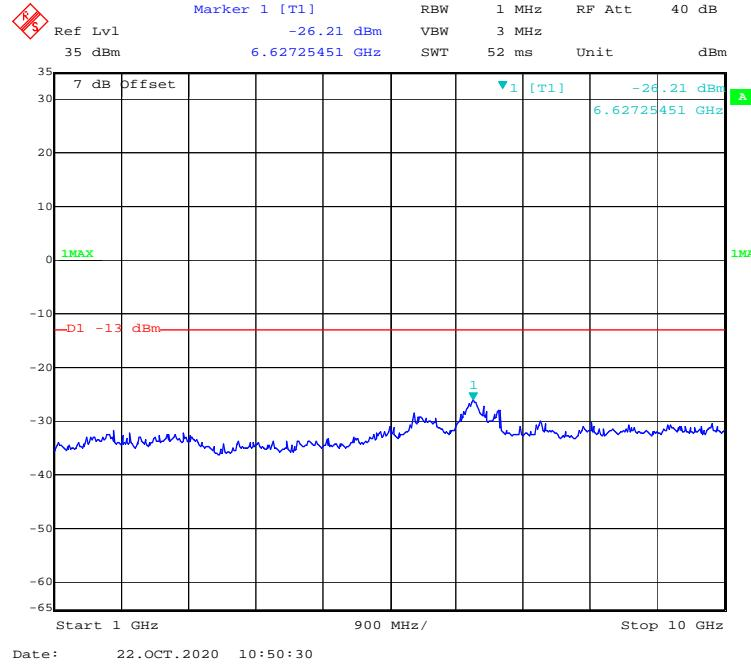
**WCDMA Band V:****30 MHz – 1GHz WCDMA (Rel 99) Mode, Low channel**
