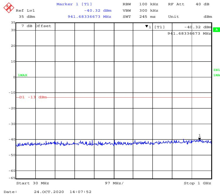
**1 GHz – 20 GHz (10 MHz, QPSK, Low Channel)**
