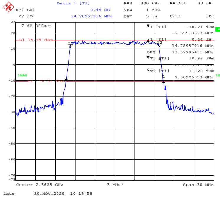
**16-QAM (20 MHz) - 99% Occupied & 26 dB Emissions Bandwidth, Low channel**
