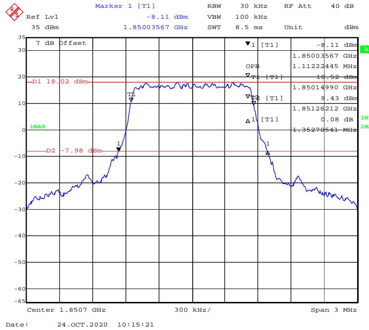
**16-QAM (3 MHz) - 99% Occupied & 26 dB Emissions Bandwidth, Low channel**
