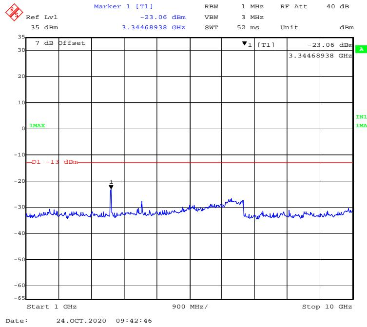
**30 MHz – 1GHz WCDMA (HSUPA) Mode, Middle channel**
