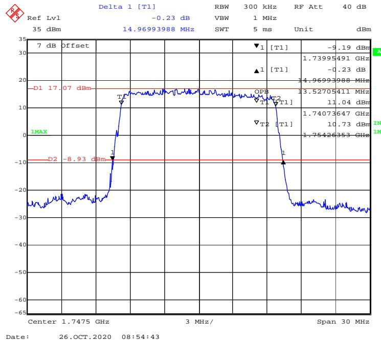
**QPSK (20 MHz) - 99% Occupied & 26 dB Emissions Bandwidth, High channel**
