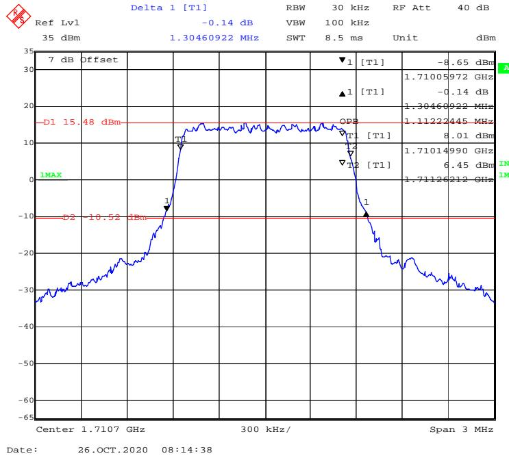
**16-QAM (3 MHz) - 99% Occupied & 26 dB Emissions Bandwidth, Low channel**
