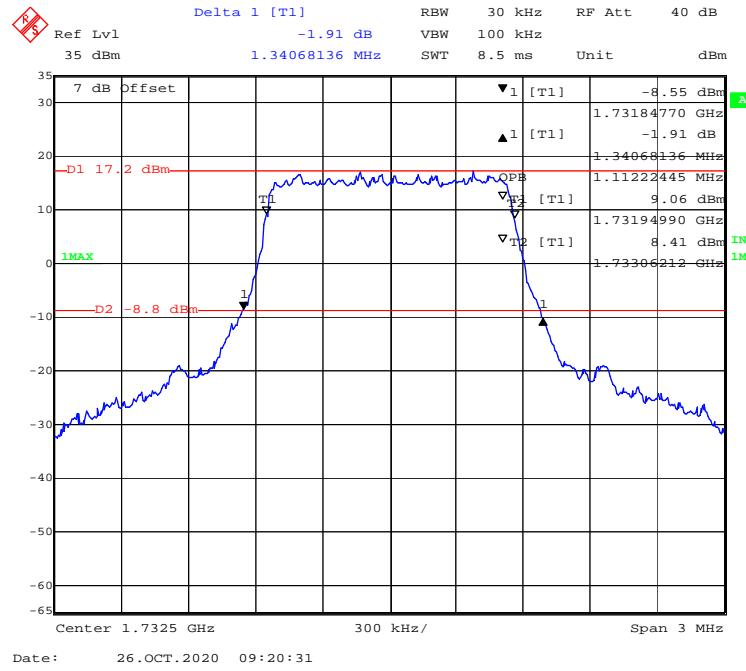
**16-QAM (3 MHz) - 99% Occupied & 26 dB Emissions Bandwidth, Middle channel**
