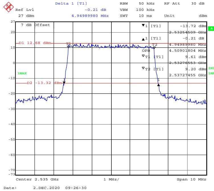
**16-QAM (10 MHz) - 99% Occupied & 26 dB Emissions Bandwidth, Middle channel**
