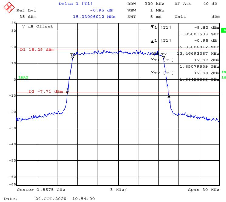
**QPSK (20 MHz) - 99% Occupied & 26 dB Emissions Bandwidth, Low channel**
