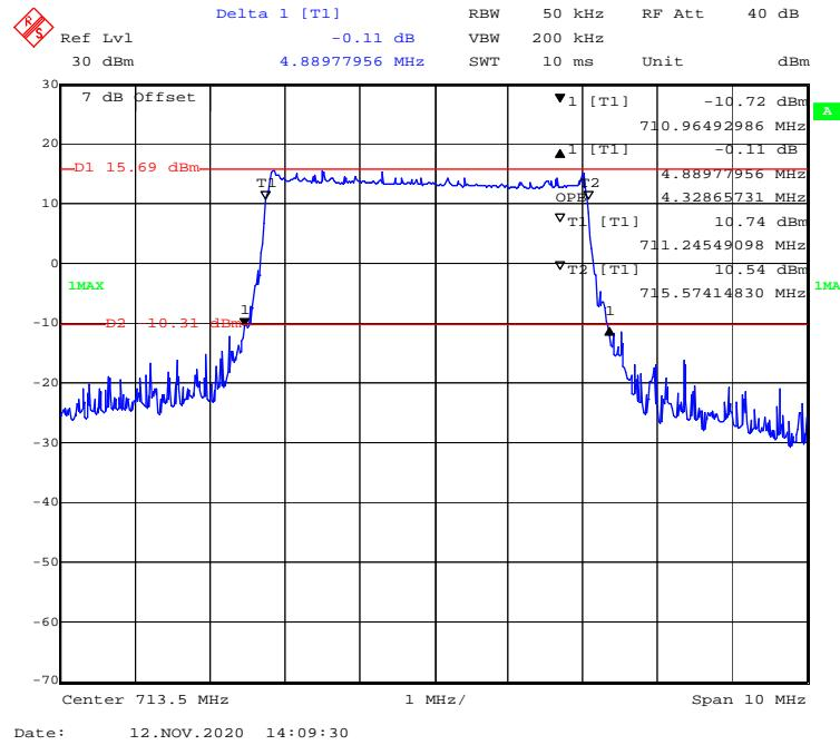
**16-QAM (10 MHz) - 99% Occupied & 26 dB Emissions Bandwidth, High channel**
