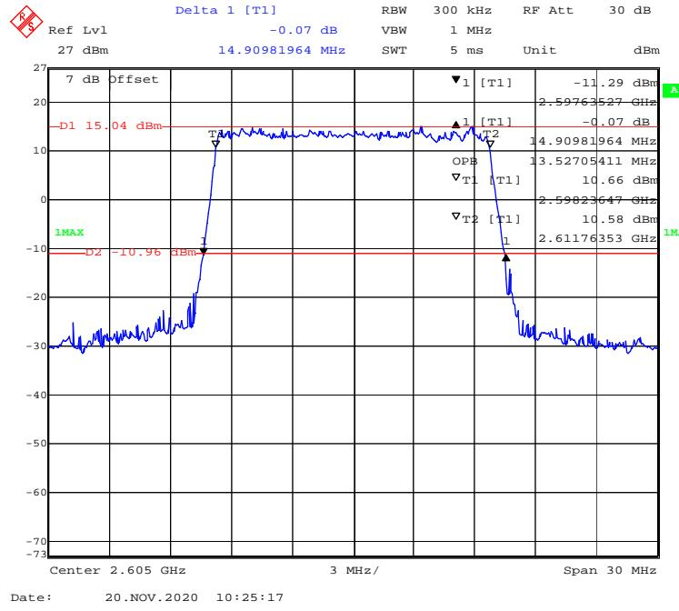
**16-QAM (20 MHz) - 99% Occupied & 26 dB Emissions Bandwidth, Middle channel**
