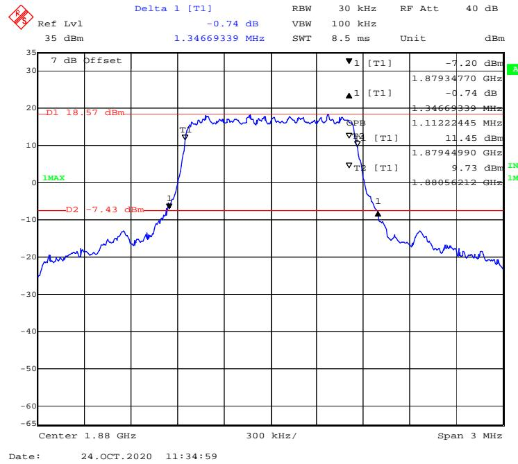
**16-QAM (3 MHz) - 99% Occupied & 26 dB Emissions Bandwidth, Middle channel**
