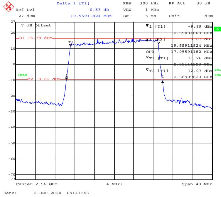
**16-QAM (5 MHz) - 99% Occupied & 26 dB Emissions Bandwidth, Low channel**
