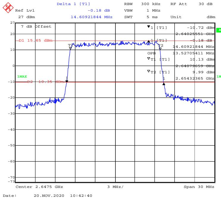
**QPSK (20 MHz) - 99% Occupied & 26 dB Emissions Bandwidth, High channel**
