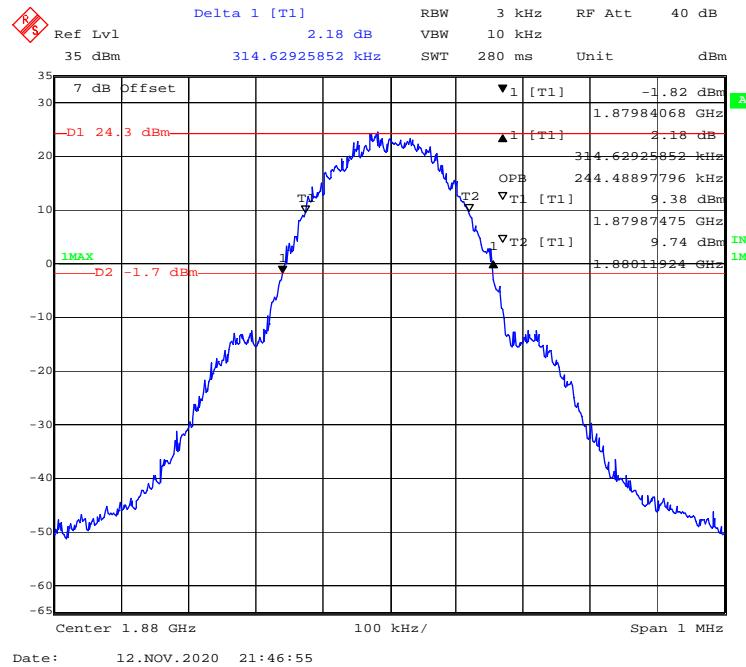
**99% Occupied & 26 dB Emissions Bandwidth for EGPRS (8PSK) High channel**
