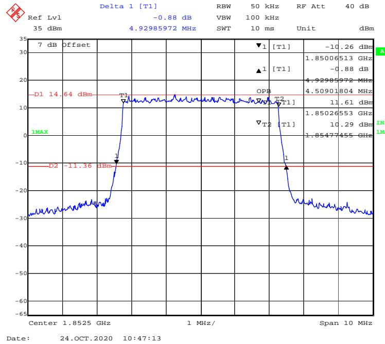
**16-QAM (10 MHz) - 99% Occupied & 26 dB Emissions Bandwidth, Low channel**
