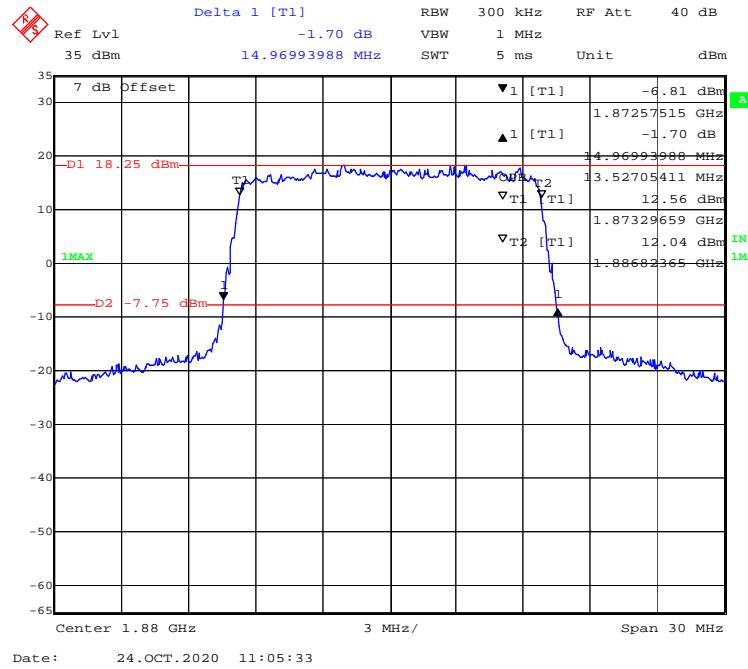
**16-QAM (20 MHz) - 99% Occupied & 26 dB Emissions Bandwidth, Middle channel**
