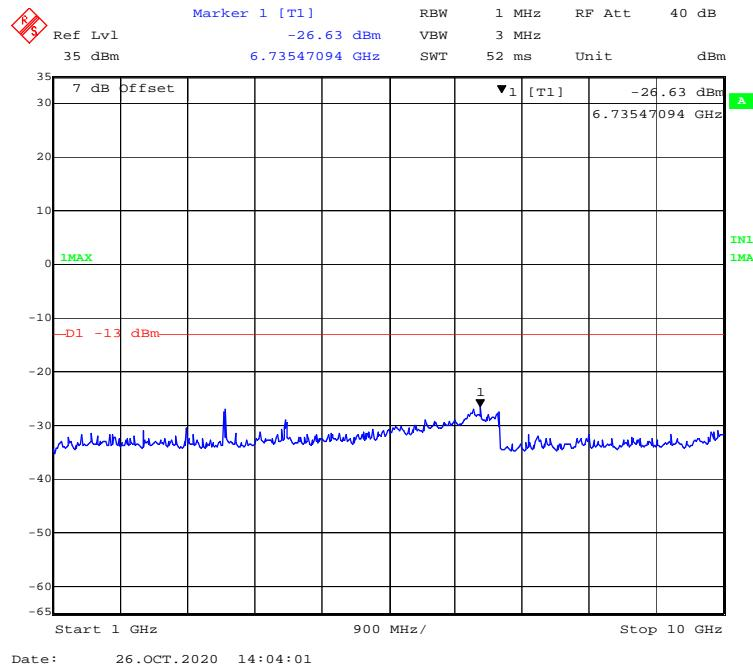
**30 MHz - 1 GHz (QPSK, 5.0 MHz, Low Channel)**
