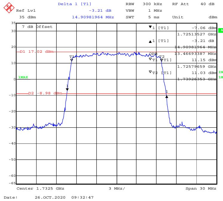
**QPSK (20 MHz) - 99% Occupied & 26 dB Emissions Bandwidth, Middle channel**
