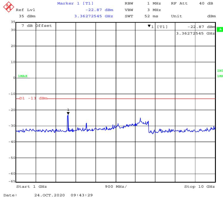
**30 MHz – 1GHz WCDMA (Rel 99) Mode, High channel**
