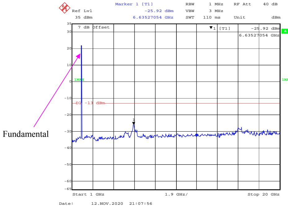
**30 MHz – 1GHz WCDMA (HSDPA) Mode , High channel**
