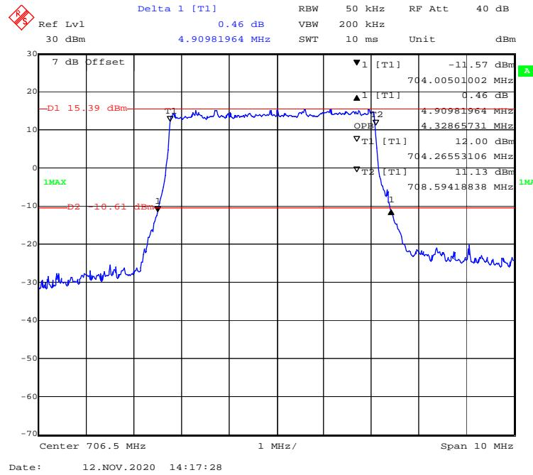
**16-QAM (10 MHz) - 99% Occupied & 26 dB Emissions Bandwidth, Low channel**
