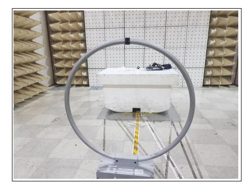
2. Photo of Radiated Spurious Emission Test (30 Mz ~ 1 000 Mz)
