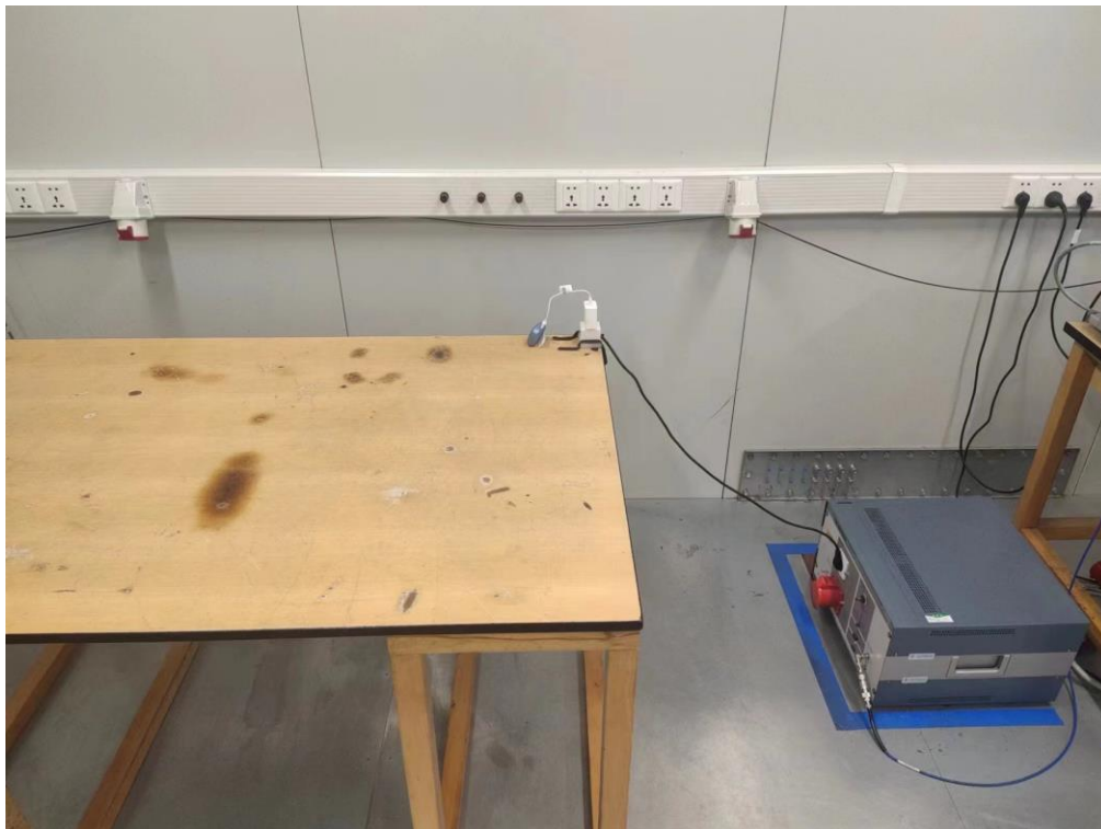
AC Conducted Emission Test Setup -Front
