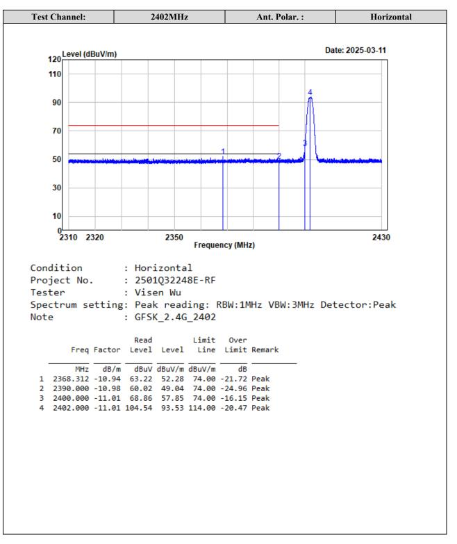
Test plots for Band Edge Measurements (Radiated):
