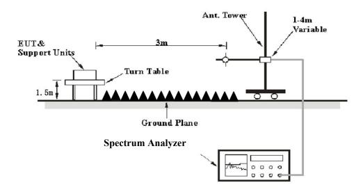
The radiated emission and out of band emission tests were performed in the 3 meters chamber test site, using the setup accordance with the ANSI C63.10-2020. The specification used was the FCC 15.209/15.205 and FCC 15.249 limits.
