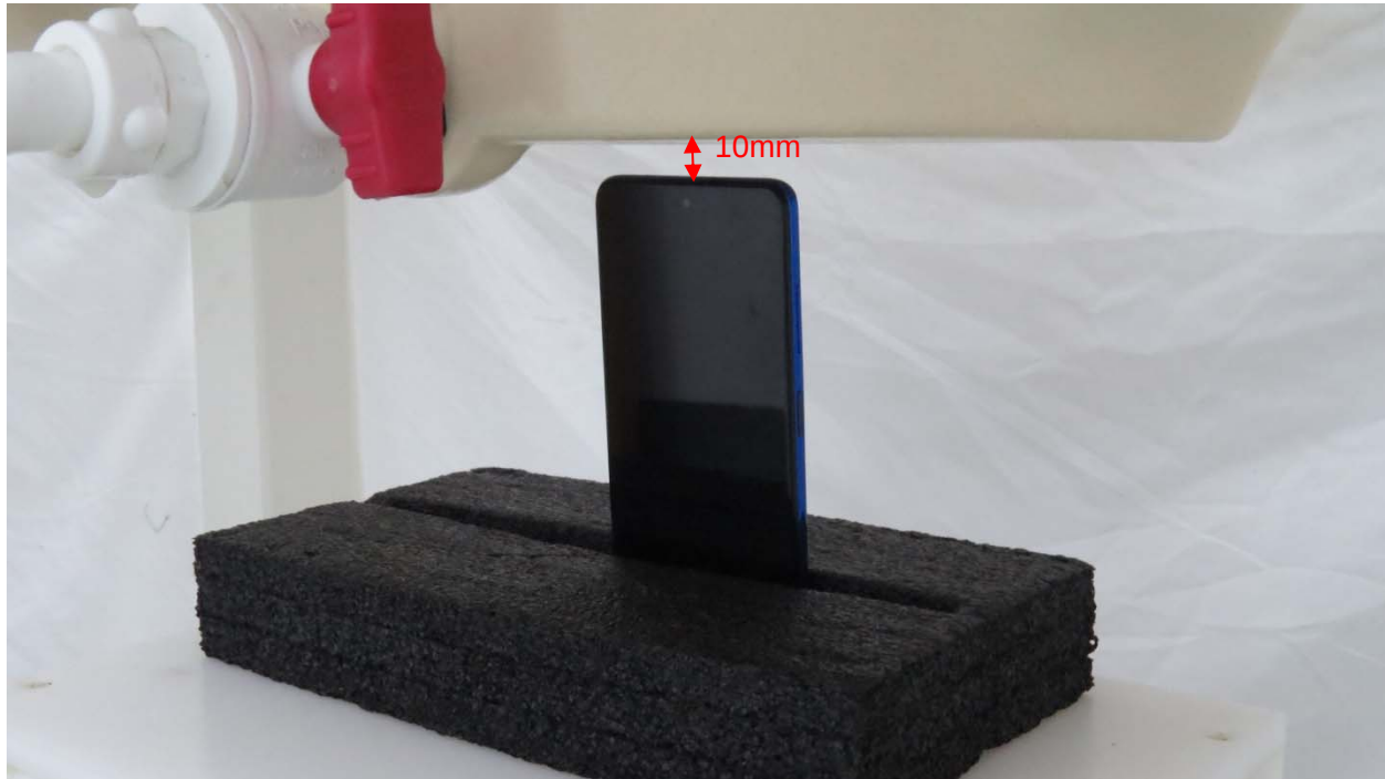
Picture 9: Top Side, the distance from handset to the bottom of the Phantom is 10mm
