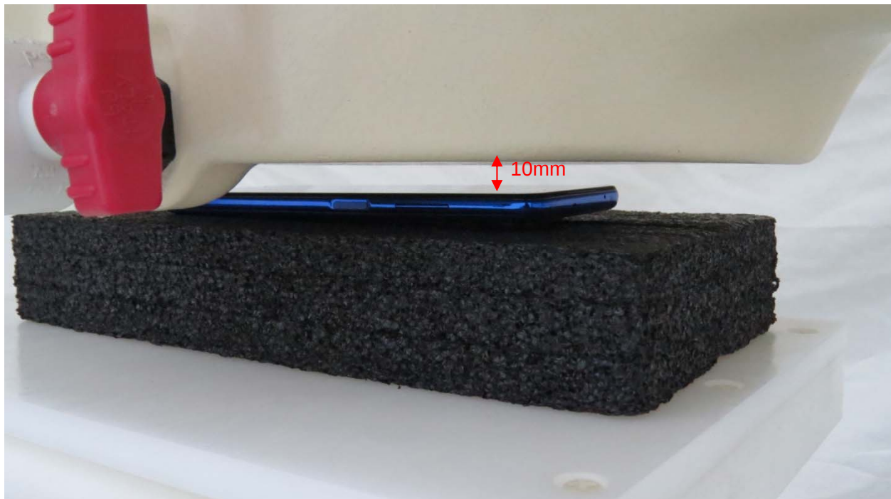
Picture 6: Front Side, the distance from handset to the bottom of the Phantom is 10mm
