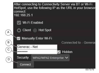
Figure 3-68. Wireless LAN Client Setup
