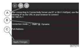
Figure 3-66. Dynamic IP Address Configuration for Ethernet
