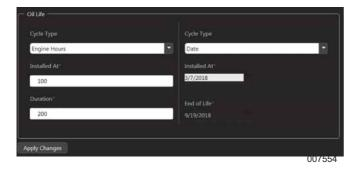
Figure 3-55. Oil Life Maintenance Setup
