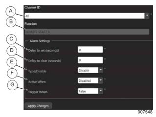
Figure 3-46. Digital Input Alarms
