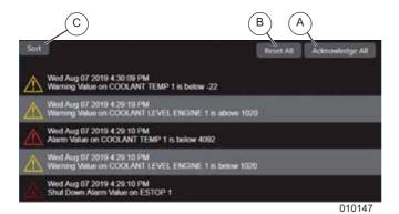
Figure 3-29. Sort, Reset and Acknowledge Alarms and Warnings
