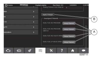
Figure 3-40. Setup Channel
