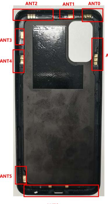
ANT ANT1:N77DRX 2G: B ANTO:GPS/ 3G: W WiFi/BT 4G: B 5G: N ANT3 ANT7:B41/N41 ANT ANT7 +N77 DRX ANT6: 2G: B5/8 TRX 3G: B5 TRX 4G: B5/12/13/17/26/71 TRX 5G: B5/71 TRX
