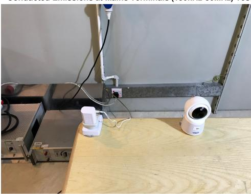
Radiated Emissions (30MHz-1GHz) Test Setup
