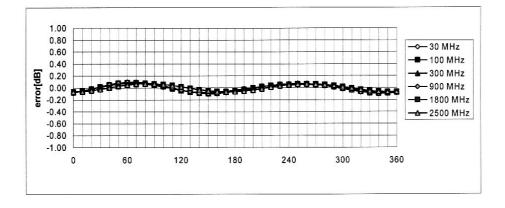
Axial Isotropy Error < ± 0.2 dB
