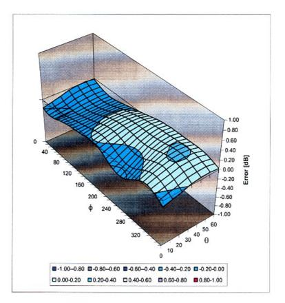
Spherical Isotropy Error < ± 0.4 dB
