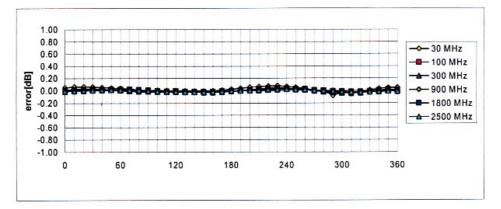
Axial Isotropy Error < ± 0.2 dB
