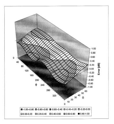
Spherical Isotropy Error < ± 0.4 dB
