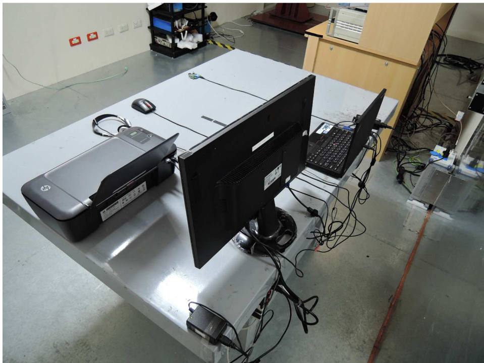
Photograph 5: Set-up for for Mains Conducted testing Back
