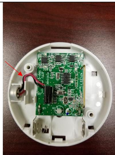
Microphone extended with wires and rubber spacer wrapped around mic.
