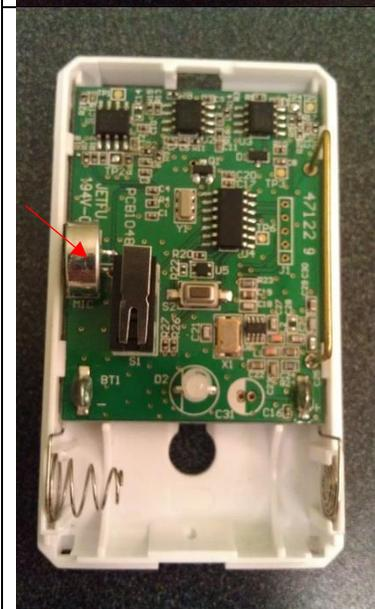
Microphone soldered directly on
