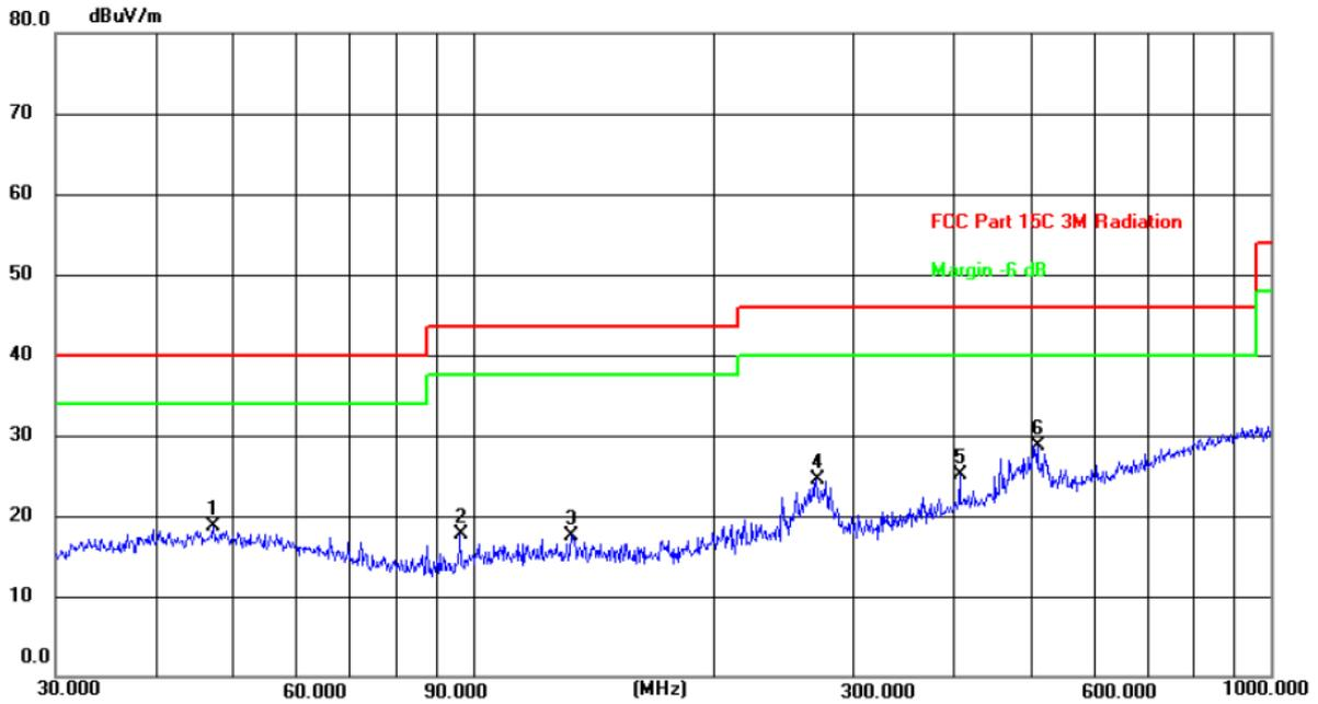
Site: Polarization: **Vertical** Temperature: 25(C)
