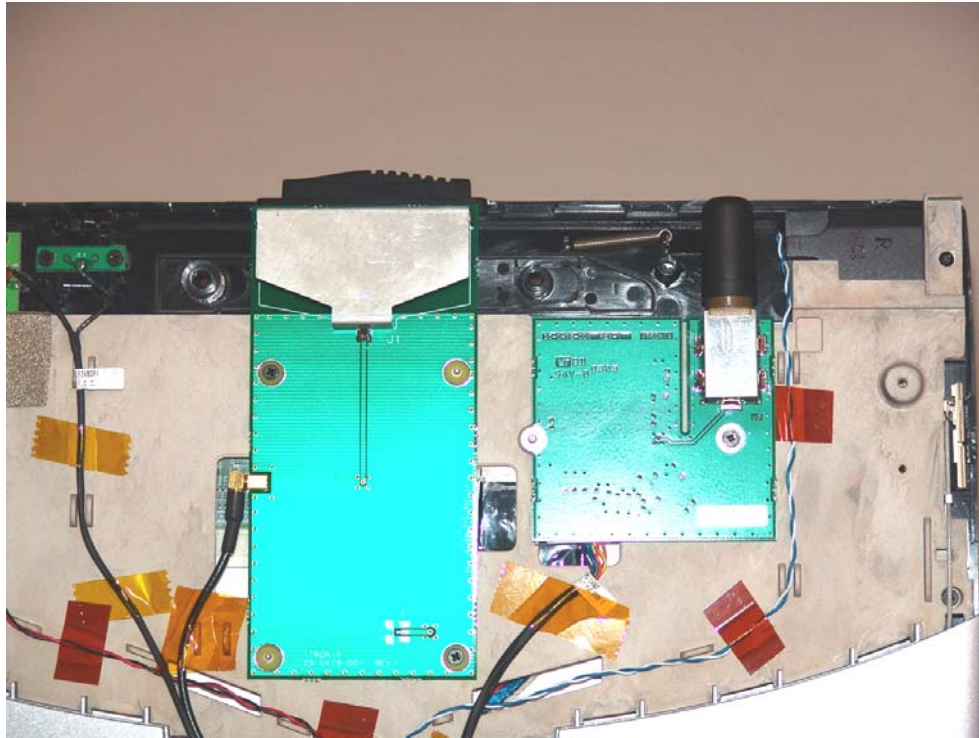
IX600 close up WAN antenna centered - GPS antenna on right side
