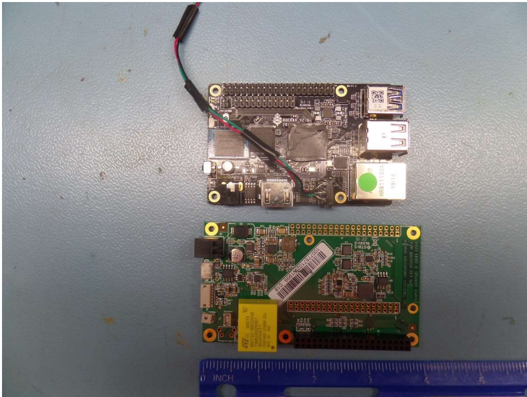
Figure 16: NP10 PAB w/HUB SOM module Rock 64 & Light and sounder board top side
